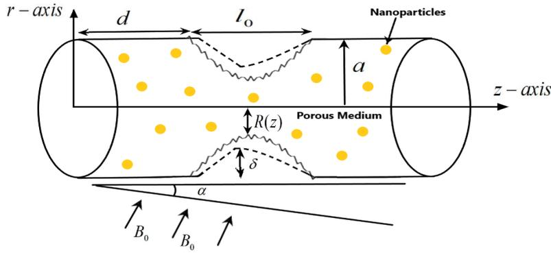
Fig. 1: Geometry of the stenosis artery
