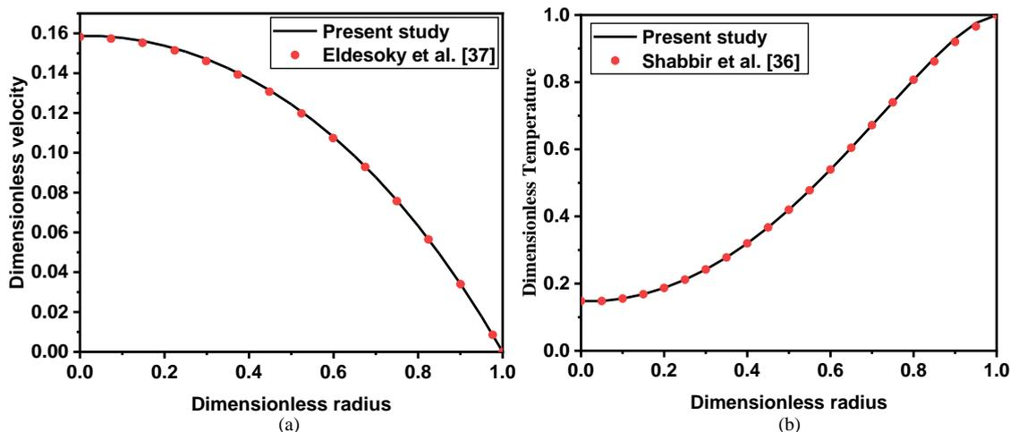
Fig 3: Comparison results for (a) dimensionless velocity profile (b) dimensionless temperature profile
