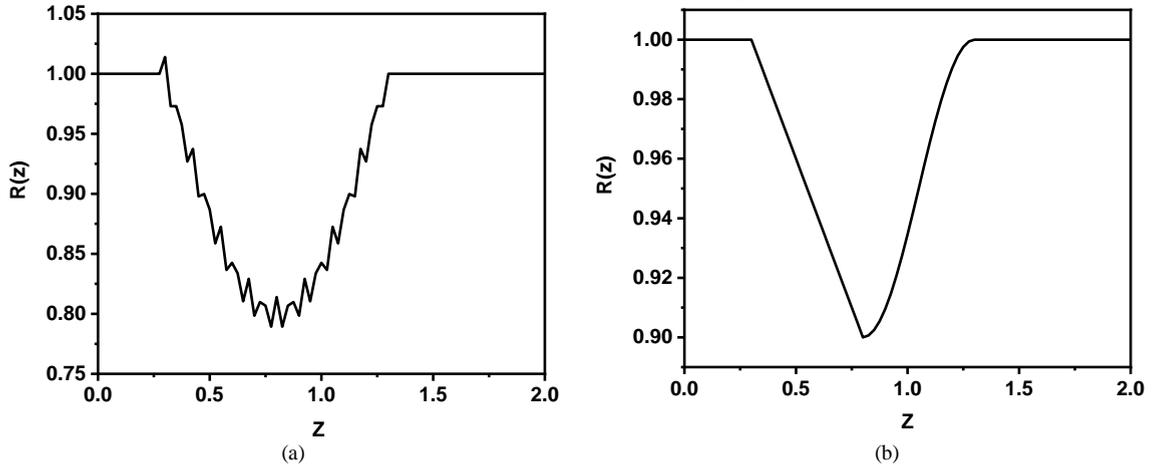
Fig 2: Representation of the shape of the stenosis (a) Irregular stenosis, (b) Composite stenosis
