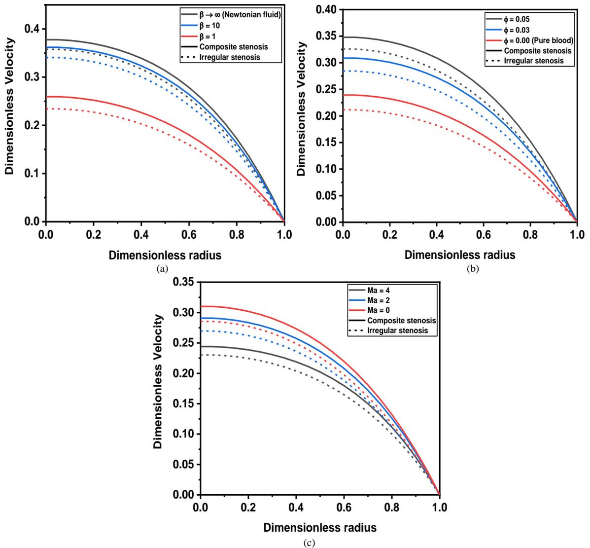
Fig 4: Effect of (a) Casson parameter  $\beta$  (b) Nanoparticle volume fraction (c) Magnetic parameter on velocity profile
