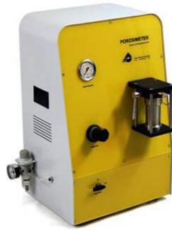
**Figure 2.** A schematic of helium porosimeter device.
