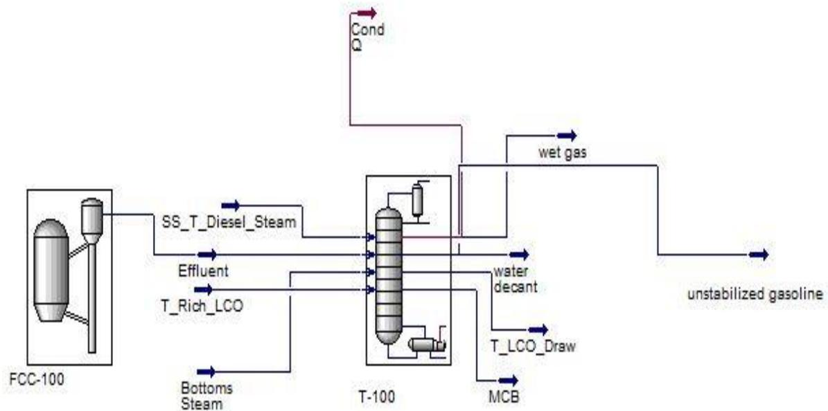
**Fig. 1.** Simulation diagram of Fluid Catalytic Cracking Unit.
