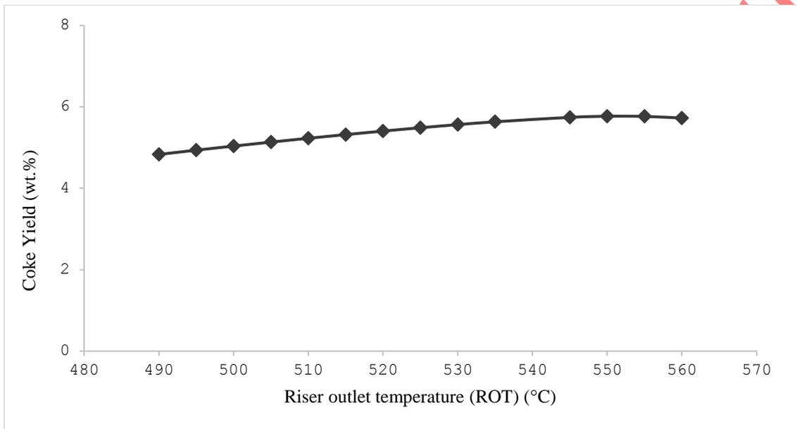
**Fig. 3.** Variation of coke with riser outlet temperature (ROT)
