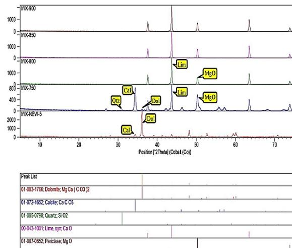
**Figure 4.** XRD pattern of the calcination of the composite sample at different temperatures.
