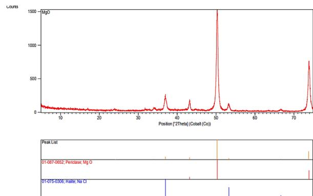
**Figure 11.** The XRD patterns of magnesium oxide.
