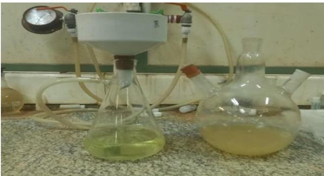
**Figure 7.** Filtration of the hydrochloric acid leachate.
