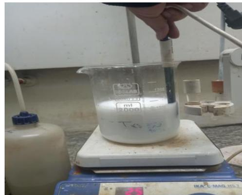
**Figure 9.** Precipitation solution of magnesium hydroxide.
