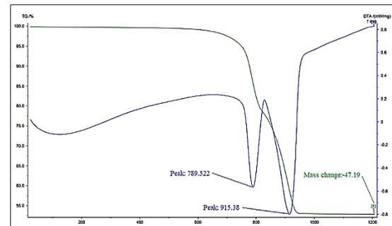
**Figure 3.** TGA-DTA diagram of the combined sample of five sampling stations.
