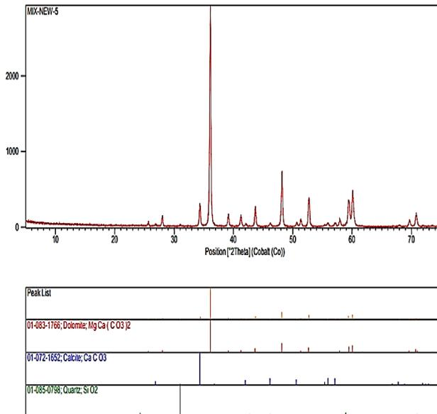
**Figure 1.** XRD diagram of the combined sample of five sampling stations.
