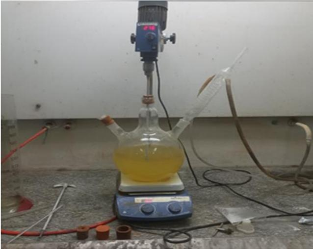
**Figure 6.** Hydrochloric acid leaching of calcined dolomite.
