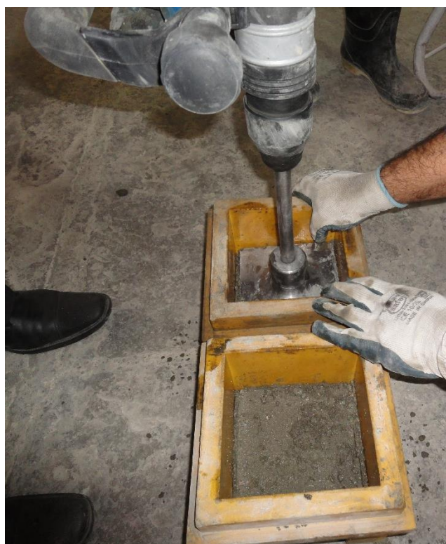
Figure 2. Molding and compaction of concrete specimens
