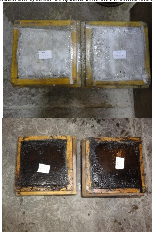
Figure 3. RCC specimens cured with different materials
