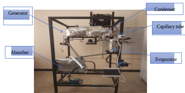
Figure 7. Absorption system cycle
