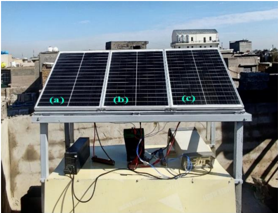
Figure 1. Experimental setup of the solar PV system (a) uncoated PV module, (b) TiO 2 -coated PV module, and (c) SiO 2 -coated PV module
