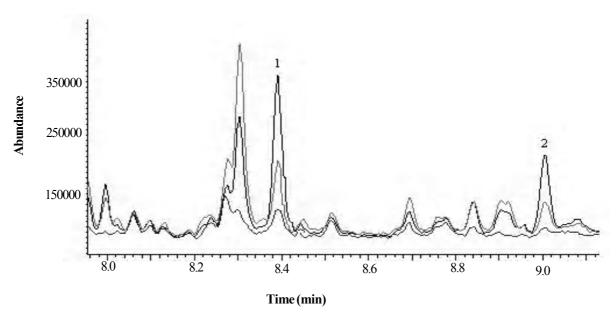
Fig. 5. GC-MS chromatograms of spiked water at 200, 100 and 50  $\mu$ g/L concentrations of endosulfan. (1)  $\alpha$ -endosulfan, (2)  $\beta$ -endosulfan
