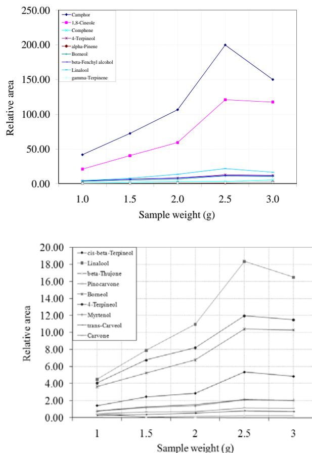
**Figure 4. Effect of sample weight on extraction efficiency. Extraction conditions: microdrop volume, 1.0  $\mu$ l; extraction time, 4 min.**
