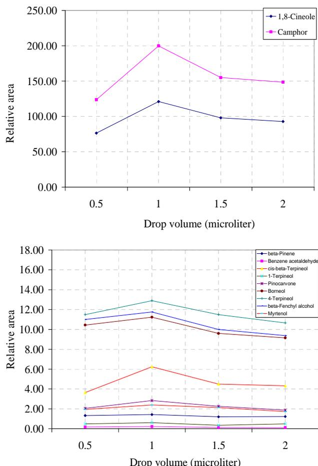
**Figure 5.** Effect of drop volume on the extraction efficiency. Extraction conditions: sample weight, 2.5 g; extraction time, 4 min.
