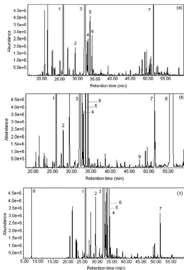
**Figure 11.** Total Ion Chromatograms of essential oil components of *Artemisia Haussknechtii* Boiss., extracted by a) hydro-distillation, b) HD-SHLPME, c) HD-DHLPME 1) 1,8-Cineole, 2) Linalool, 3) Camphor, 4) Borneol, 5) 4-Terpineol, 6) *beta*-Fenchyl alcohol, 7) *cis*-Davanone, 8) Solvent, and 9) Internal standard.
