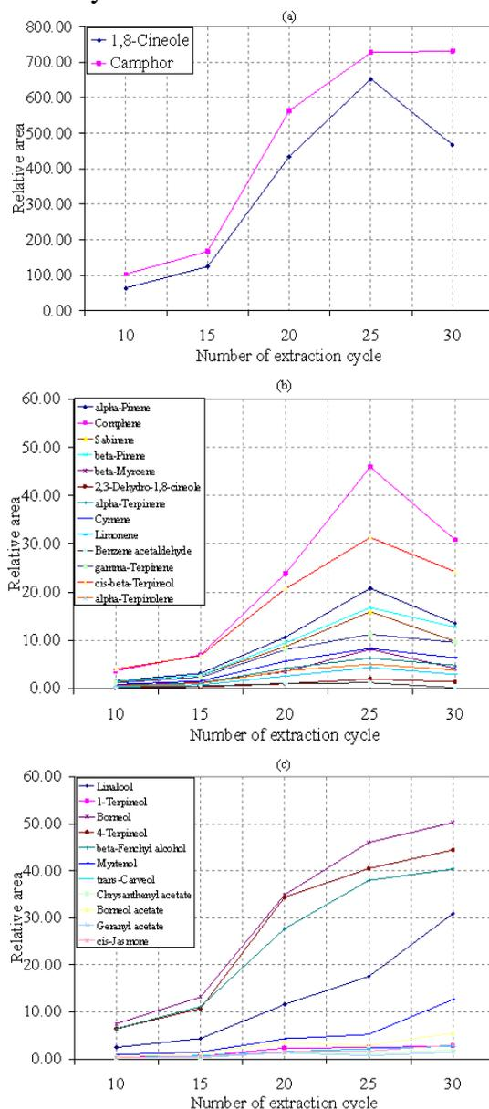
**Figure 10. a, b and c- Effect of number of extraction cycle on the extraction efficiency. Extraction conditions: sampling volume, 4.0  $\mu\text{l}$ ; withdrawal rate, 1.0  $\mu\text{l/s}$ ; solvent volume, 1.0  $\mu\text{l}$ .**
