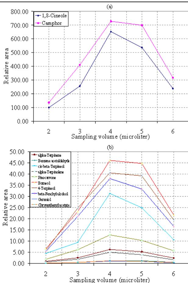
**Figure 7.** Effect of sampling volume on the extraction efficiency. Extraction conditions: solvent volume, 1.0  $\mu\text{l}$ ; withdrawal rate, 1.0  $\mu\text{l/s}$ ; extraction cycles, 25
