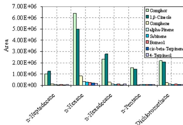
**Figure 6.** Effect of various solvents on the extraction efficiency. Extraction conditions: sample weight, 2.5g; extraction cycles, 25; sampling volume, 4  $\mu$ l; solvent volume, 1  $\mu$ l; withdrawal rate, 1  $\mu$ l/s.
