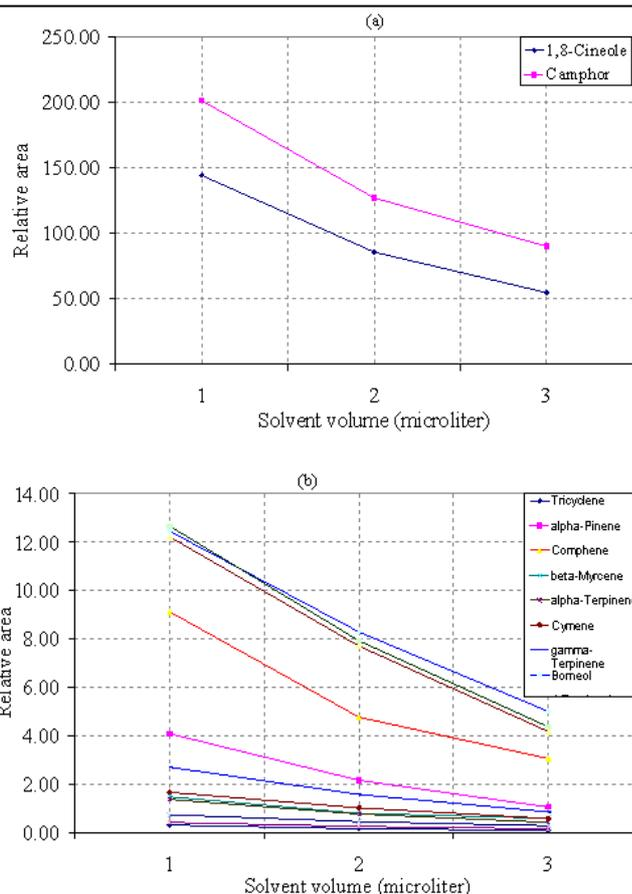
**Figure 8.** Effect of solvent volume on the extraction efficiency. Extraction conditions: sampling volume, 4.0  $\mu\text{l}$ ; syringe withdrawal rate, 1.0  $\mu\text{l/s}$ ; extraction cycles, 25.
