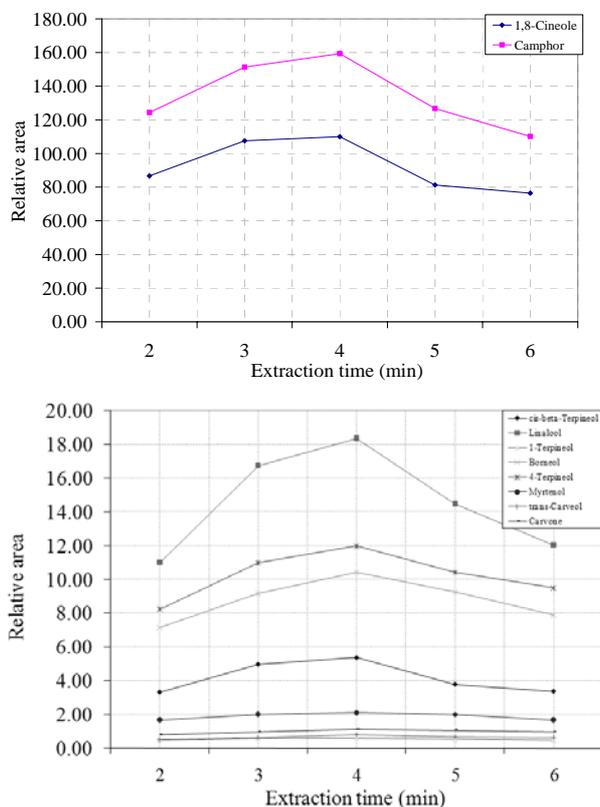
**Figure 3. Effect of extraction time on the efficiency. Extraction conditions: sample weight, 2.5 g; microdrop volume, 1.0  $\mu$ l.**
