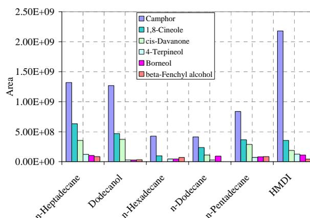
**Figure 2.** Relative extraction efficiency for different solvents.
