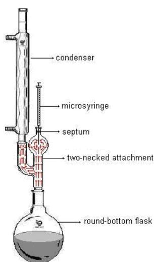
**Figure 1.** The HD-DHLPME apparatus with schematic diagram of flowing vapor.
