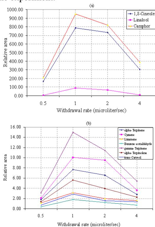
**Figure 9. Effect of syringe withdrawal rate on the extraction efficiency. Extraction conditions: sampling volume, 4.0  $\mu\text{l}$ ; solvent volume, 1.0  $\mu\text{l}$ ; extraction cycles, 25.**
