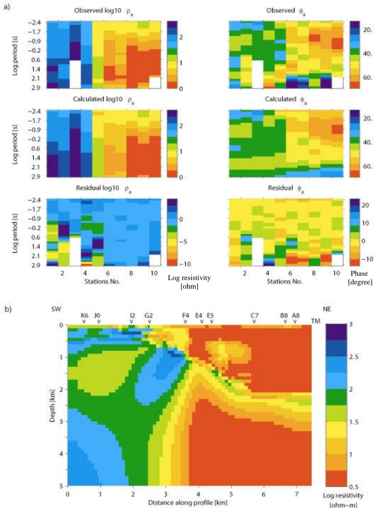
Figure 11. TM-model and datafit for profile 1.
