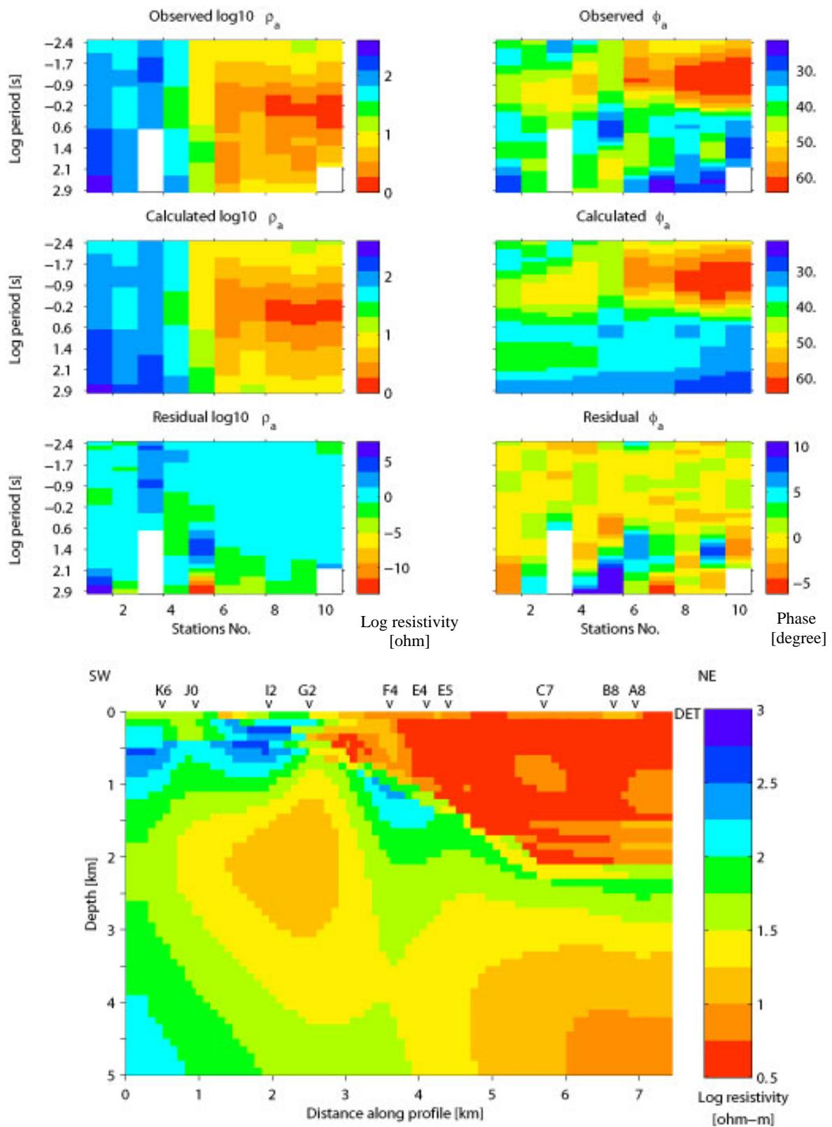
Figure 12. DET-model and datafit for profile 1.
