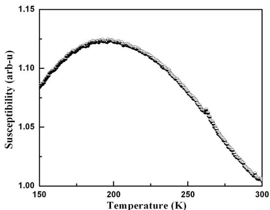
**Figure 9.** Temperature dependence of the real part of AC susceptibility for the  $\text{MgFe}_2\text{O}_4/\text{MWCNTs}$  nanocomposites calcined in Ar at  $600\text{ }^\circ\text{C}/2\text{h}$ . The applied field is  $800\text{ A/m}$ .
