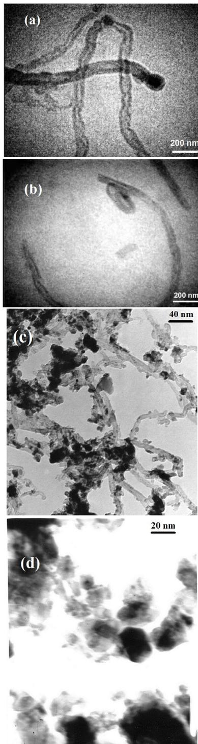
**Figure 6.** TEM images of (a) the pristine MWCNTs, (b) MWCNTs after acid treatment, (c) the MgFe<sub>2</sub>O<sub>4</sub>/MWCNTs nanocomposites calcined in Ar at 600 °C/2h and (d) MgFe<sub>2</sub>O<sub>4</sub> nanoparticles calcined in Ar at 600 °C/2h.
