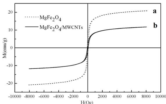
**Figure 8.** Hysteresis loops of (a)  $\text{MgFe}_2\text{O}_4$  nanoparticles and (b) the  $\text{MgFe}_2\text{O}_4/\text{MWCNTs}$  nanocomposites calcined in Ar at  $600\text{ }^\circ\text{C}/2\text{h}$ .
