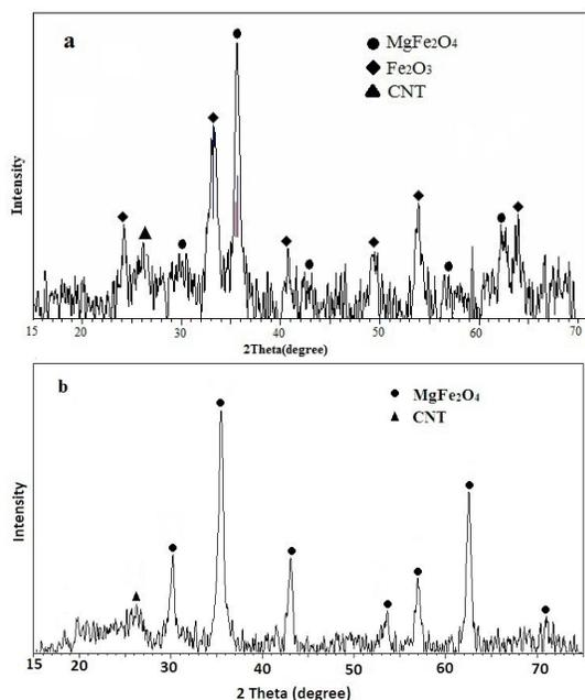
Figure 5. XRD patterns of the  $\text{MgFe}_2\text{O}_4/\text{MWCNTs}$  nanocomposites calcined in Ar at (a)  $475\text{ }^\circ\text{C}/2\text{h}$  and (b)  $600\text{ }^\circ\text{C}/2\text{h}$ .
