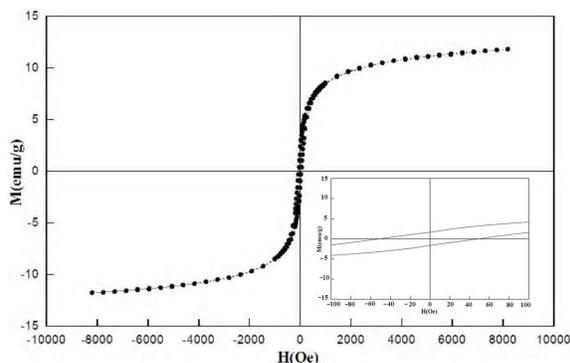
**Figure 7.** Hysteresis loop of the  $\text{MgFe}_2\text{O}_4/\text{MWCNTs}$  nanocomposites calcined in Ar at  $600\text{ }^\circ\text{C}/2\text{h}$ .
