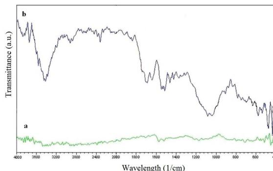
**Figure 1.** FT-IR spectra of (a) Pristine MWCNTs (b) opened MWCNTs.
