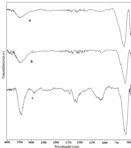
**Figure 2.** FT-IR spectrum of (a) the  $\text{MgFe}_2\text{O}_4$  nanoparticles calcined in Ar at 600 °C/2h. The  $\text{MgFe}_2\text{O}_4/\text{MWCNTs}$  nanocomposites calcined in Ar at (b) 475 °C/2h and (c) 600 °C/2h.
