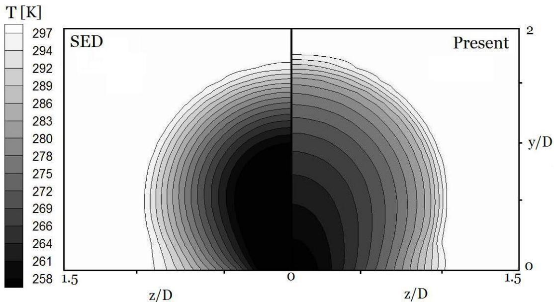
Fig. 12. Temperature contours in the y-z plane, at x/D=10: comparison between SED and present model.
