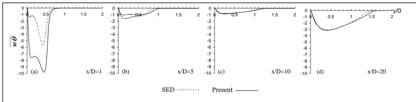
Fig. 10. Spanwise turbulent heat flux distributions at the center-line plane: comparison of SED with the present first-moment closure.
