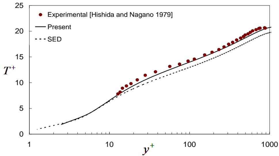
Fig.4. Normalized means temperature profiles in wall coordinates
