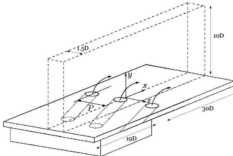
Fig. 2. Schematic of the experimental setup [Sinha et al., 1991, [22]] and computational domain.
