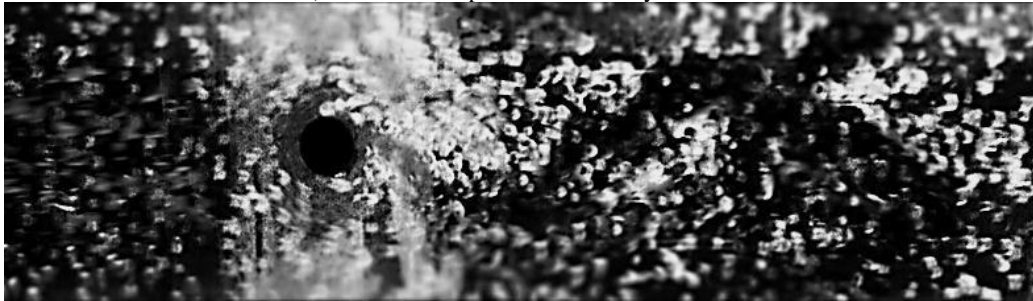
c) Photo of air- water flow around a cylindrical tube.
