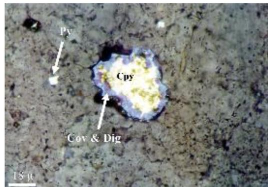
**Figure 12.** Photomicrograph of disseminated fine-grained anhedral chalcopyrite in inner parts of altered zones, reflected light, oil, PPL.
