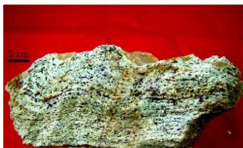
**Figure 5.** Oxidized pyrites (Py I) parallel to mylonitic foliation in intensely deformed (ultramylonite) felsic schist.
