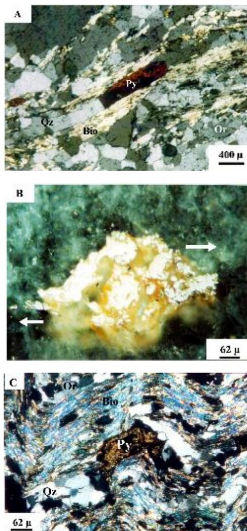
**Figure 6.** Photomicrographs of pyrite (Py I). A: a deformed and elongated euhedral oxidized pyrite perpendicular to the maximum stress axis, and parallel to mylonitic foliation, transmitting light, XPL. B: a deformed and oxidized pyrite with  $\sigma$ -type mantle-porphyroblast shape, reflected light, oil, PPL. C: a deformed and folded oxidized pyrite parallel to mylonitic foliation, transmitting light, XPL. Qz: quartz, Or: orthoclase, Bio: biotite.
