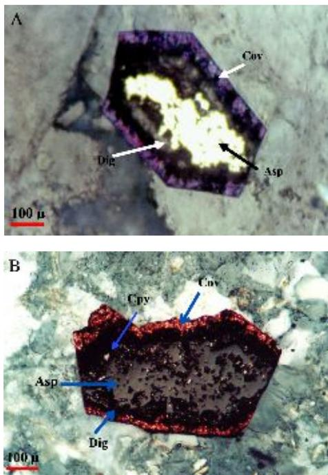
**Figure 8.** Photomicrographs of euhedral (A) and subhedral (B) arsenopyrite grains with alteration of covellite and digenite at the grain margins. Chalcopyrite inclusions (Cpy II) are observed in B. A: reflected light, oil, PPL and B: reflected light, oil, XPL. Asp: arsenopyrite, Cpy: chalcopyrite, Dig: digenite, Cov: covellite.
