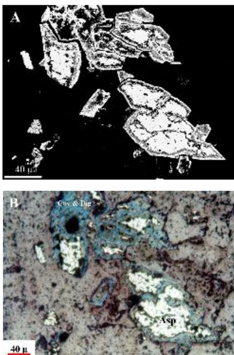
**Figure 9.** Back-scattered electron (A) and reflected light, oil, PPL (B) images showing arsenopyrite aggregates in deformed and altered rocks from brittle shear zone.
