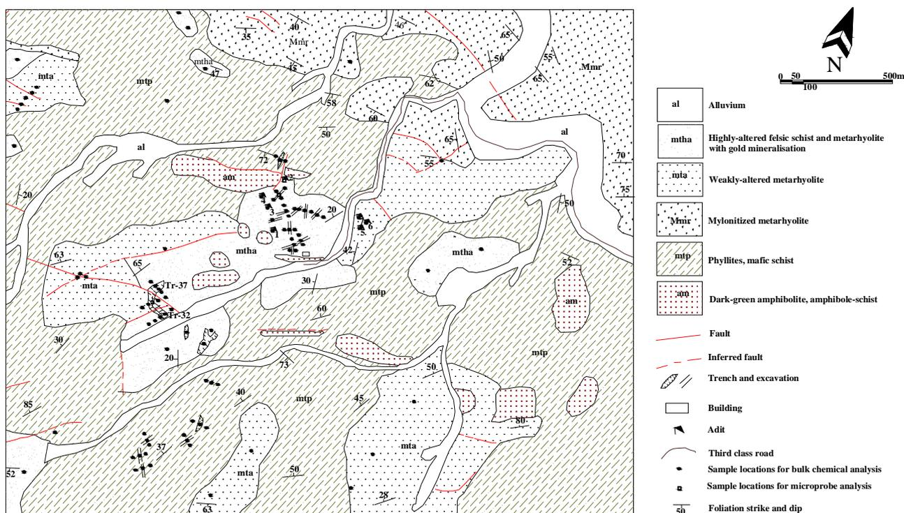
**Figure 4.** Geological map and location of tunnels, trenches and samples at the Chah-Bagh gold occurrence [8].
