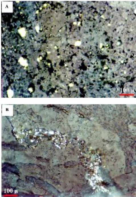
**Figure 7.** Photomicrographs of disseminated (A) and veinlet (B) fine-grained anhedral to subhedral pyrite (Py II) in inner parts of altered zones, reflected light, PPL.
