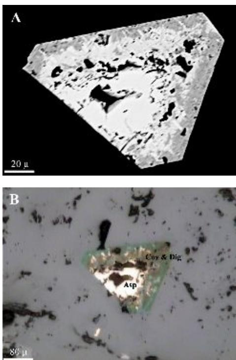
**Figure 10.** Back-scattered electron (A) and reflected light, oil, PPL (B) images showing arsenopyrite (Asp) replaced by covellite (Cov) and digenite (Dig).
