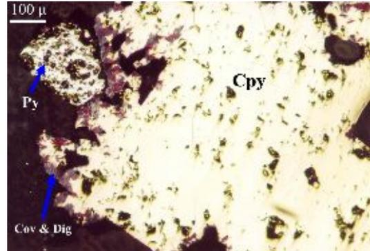
**Figure 11.** Photomicrograph of chalcopyrite (Cpy I) in close association with grains of pyrite (Py I), reflected light, oil, PPL. Py: pyrite, Cpy: chalcopyrite, Dig: digenite, Cov: covellite.
