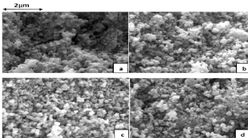
**Fig. 1.** SEM micrographs of fractured surface of (a) undoped SnO<sub>2</sub> and doped SnO<sub>2</sub> samples with (b) 10mol% ZnO; (c) 7.5mol% In<sub>2</sub>O<sub>3</sub>; (d) 10mol% ZnO - 7.5 mol% In<sub>2</sub>O<sub>3</sub>
