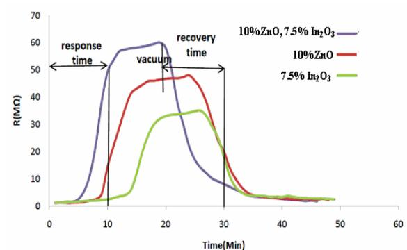
Fig. 9. Response and recovery time for ZnO and In<sub>2</sub>O<sub>3</sub> added samples.
