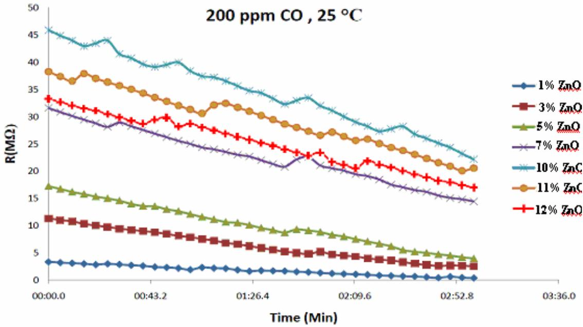
Fig. 6. Variation of electrical resistivity of ZnO doped SnO<sub>2</sub> samples with time in 200 ppm CO at 25°C
