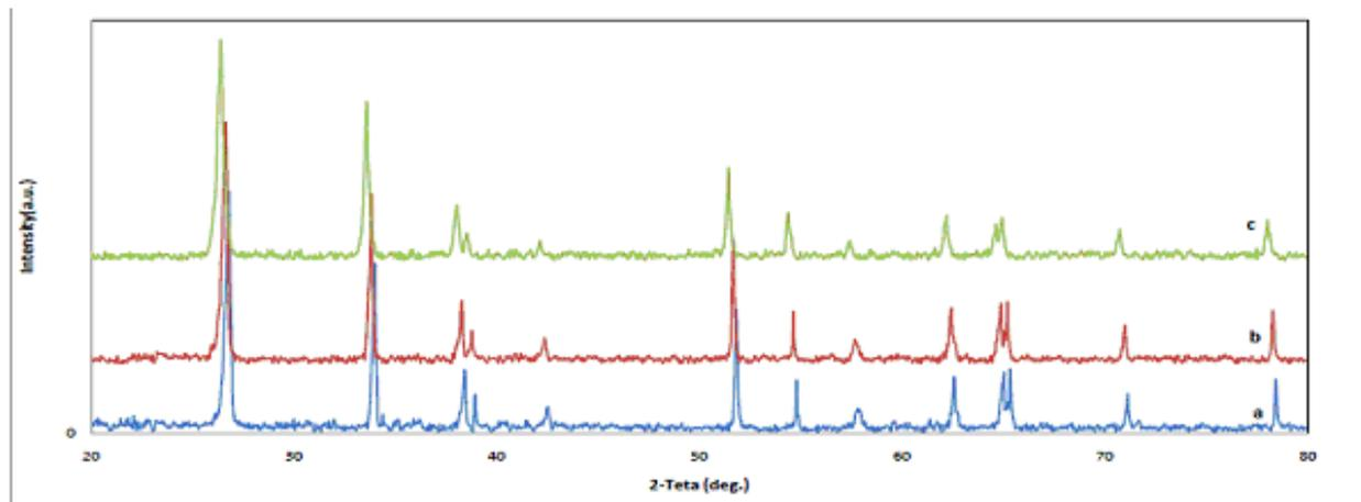
**Fig. 4.** XRD patterns of: (a) pure SnO<sub>2</sub> and SnO<sub>2</sub> samples with (b) 1 mol% and (c) 3 mol% In<sub>2</sub>O<sub>3</sub>
