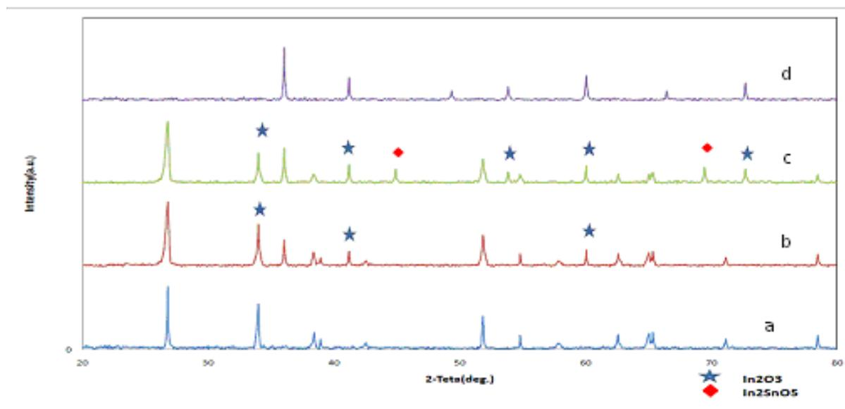
**Fig. 5.** XRD patterns of (a) Pure SnO<sub>2</sub> and In<sub>2</sub>O<sub>3</sub> doped samples with (b) 7.5 mol% , (c) 10 mol% and (d) pure In<sub>2</sub>O<sub>3</sub>
