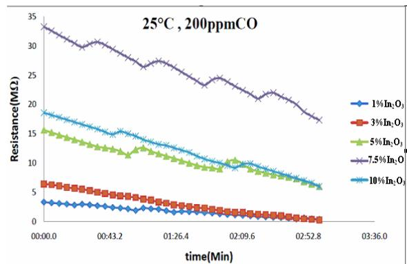
Fig. 7. Variation of electrical resistivity of nano In<sub>2</sub>O<sub>3</sub> doped SnO<sub>2</sub> samples with time in 200 ppm
