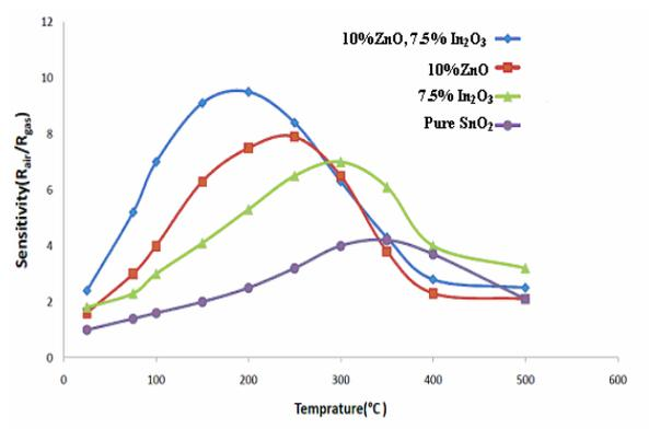
Fig. 8. The temperature dependence of the sensitivity of SnO<sub>2</sub> and ZnO/ In<sub>2</sub>O<sub>3</sub> doped SnO<sub>2</sub> to 200-ppm CO gas
