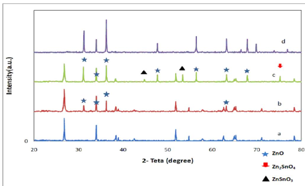
**Fig. 3.** XRD patterns of : (a) pure  $\text{SnO}_2$  ; ZnO doped  $\text{SnO}_2$  samples with (b) 10 mol% ; (c) 12 mol% and (d) pure ZnO sample
