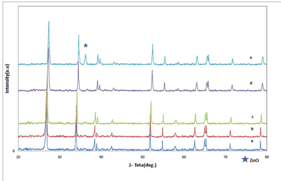
**Fig. 2.** XRD patterns of (a) pure  $\text{SnO}_2$  and ZnO doped  $\text{SnO}_2$  samples with (b) 1mol% , (c) 3mol% , (d) 5mol% and (e) 7mol%
