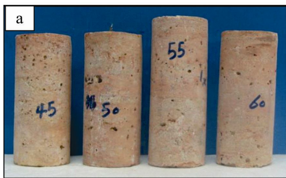
Figure 4: The change in visual appearance of Travertine-I a) before and b) after salt crystallization test
