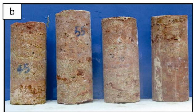
Figure 4: The change in visual appearance of Travertine-I a) before and b) after salt crystallization test
