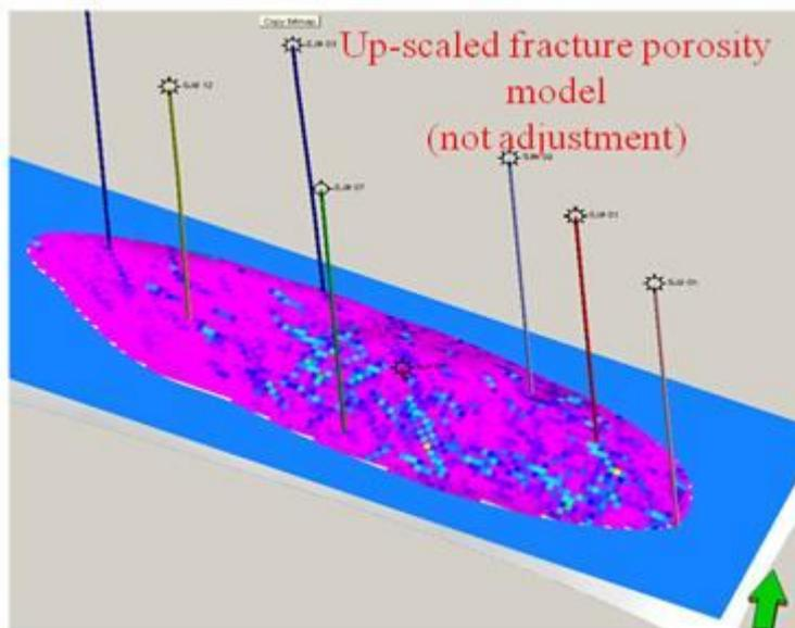
Figure 10: 3D fracture permeability in the reservoir based on DFN model
