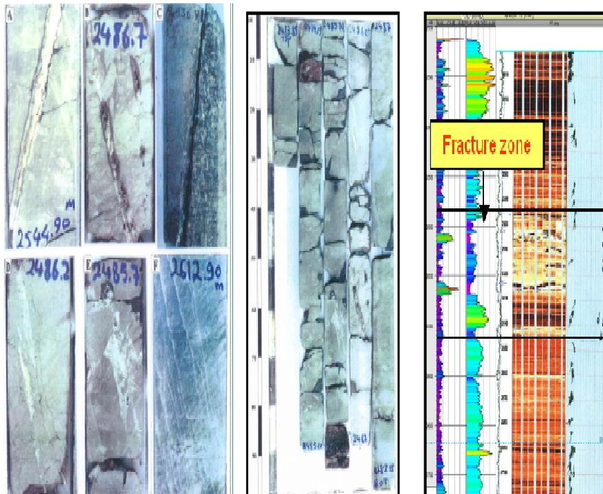
Figure 3: Core data and FMI log in the fractured reservoir
