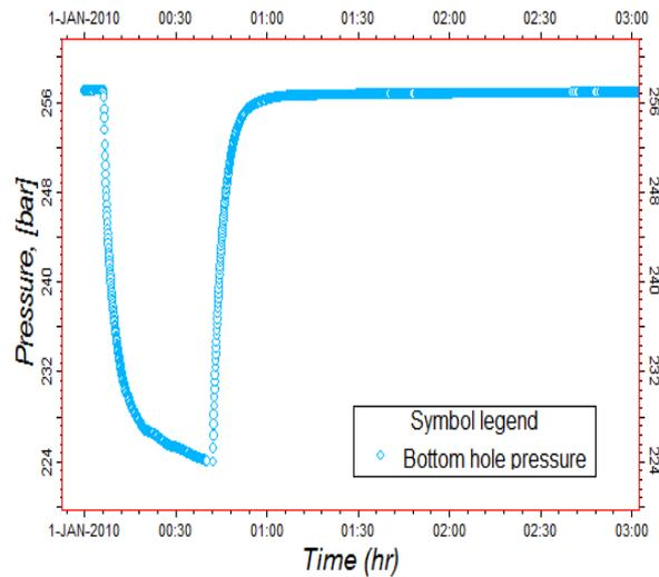
Figure 9: Observed data for a transient pressure test
