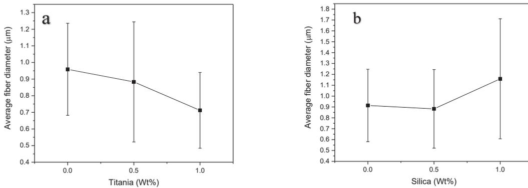
Fig. 3- Average fiber diameter of electrospun fibers at constant amount (0.5 wt%) of a) silica and b) titania.
