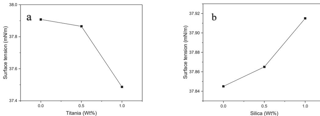
Fig. 5- Surface tension of composite polymer solutions at constant amount (0.5 wt%) of a) silica and b) titania.
