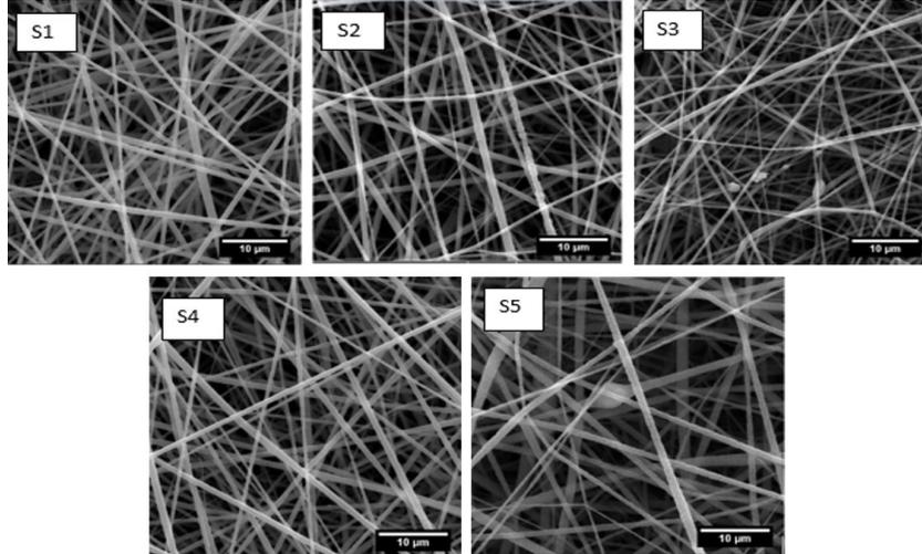
Fig. 1- SEM images of electrospun fibers.
