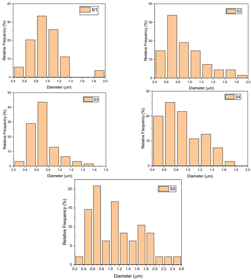
Fig. 2- The fiber diameter distribution of fibrous mats.
