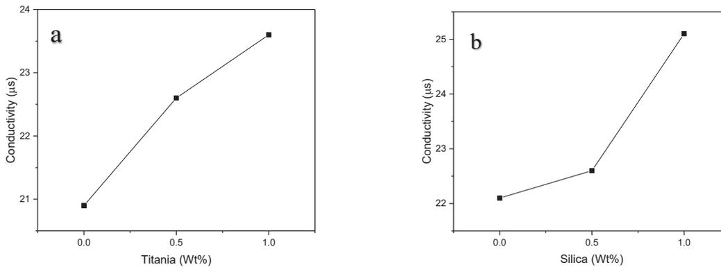
Fig. 4- Conductivity of composite polymer solutions at constant amount (0.5 wt%) of a) silica and b) titania.
