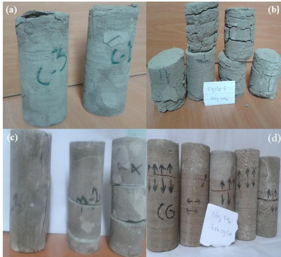
Figure 6: Selected decay phenomena occurred during salt crystallization phenomenon. a) Slaking and flaking (type C sandstone); b) loss of material, slaking and flaking (Tr type sandstone); c) and d) delamination (type A and CG sandstones)
