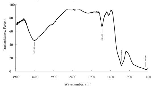
Figure 2. FT IR spectrum of the TiO<sub>2</sub>/Nd
