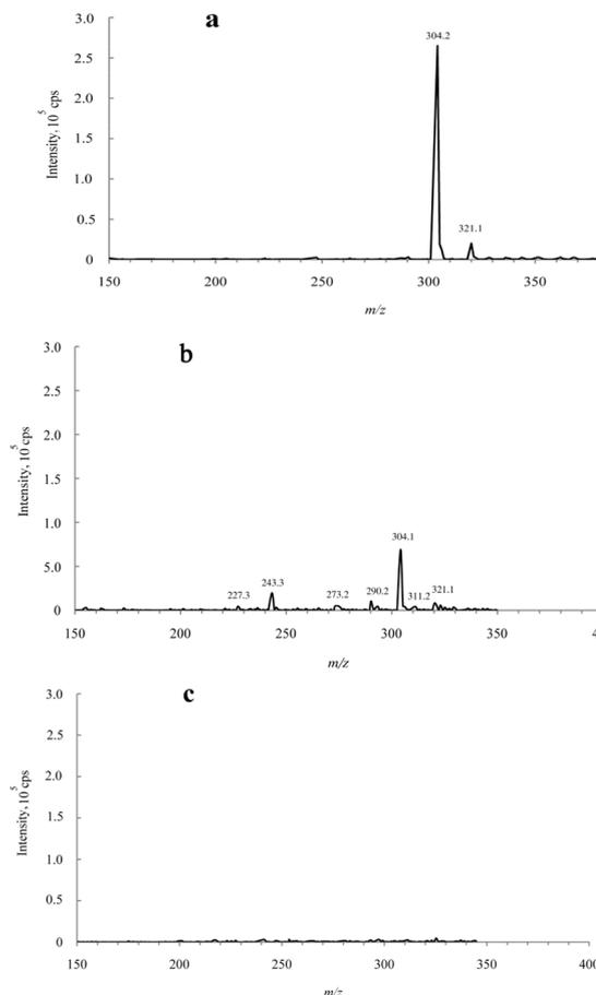
Figure 8. LC-Mass analysis of methylorange before degradation (a), after 60 min (b) and after degradation (c) by TiO<sub>2</sub>/Nd/Magnetite at pH=7
