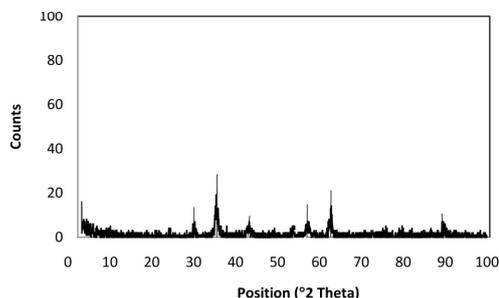
Figure 3. XRD pattern of Magnetite
