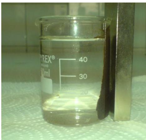
Figure 7. Catalyst separation by a magnet
