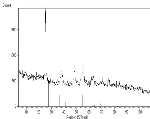
Figure 1. XRD pattern of TiO<sub>2</sub>/Nd
