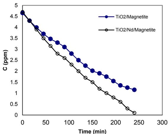
Figure 5. Comparing the photocatalytic activity of TiO<sub>2</sub>/Magnetite and TiO<sub>2</sub>/Nd/Magnetite at pH=7
