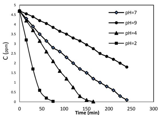
Figure 6. pH effect on degradation time by TiO<sub>2</sub>/Magnetite
