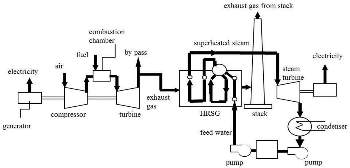
Fig. 1. Schematic view of a combined cycle
