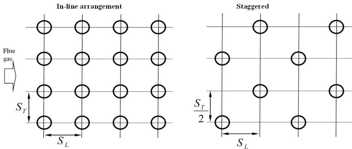
Fig. 3. Tube arrangements in HRSGs
