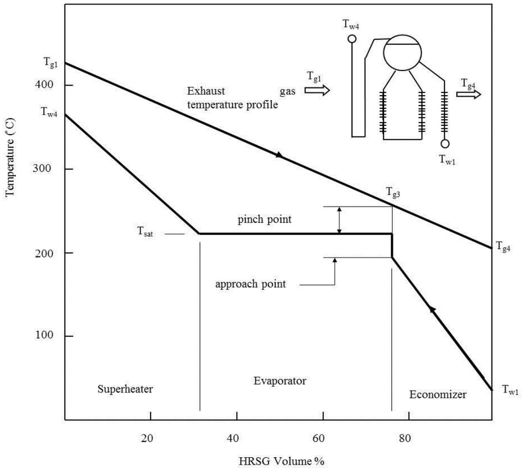
Fig. 2. A schematic view of the temperature profile in an HRSG
