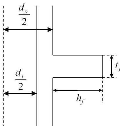
Fig. 4. A schematic sectional view of a fin with consistent thickness
