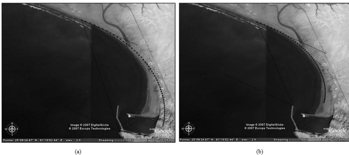
Fig. 4. Comparison between fitted parabolic model (dash-dot) and actual shape of Beris Bay, a) Before construction of the port – diffraction point at the tip of the headland, b) After construction of the port – diffraction point at the tip of the main breakwater.
