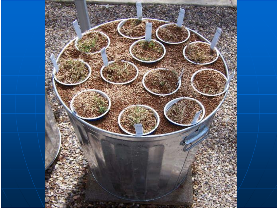
Fig. 4. Stainless steel galvanized can (one replication of the plant) containing 150 kg fritted clay and the cups just planted with saltgrass ( Distichlis spicata ) at the beginning of the plant establishment stage (Pessarakli, 2011)
