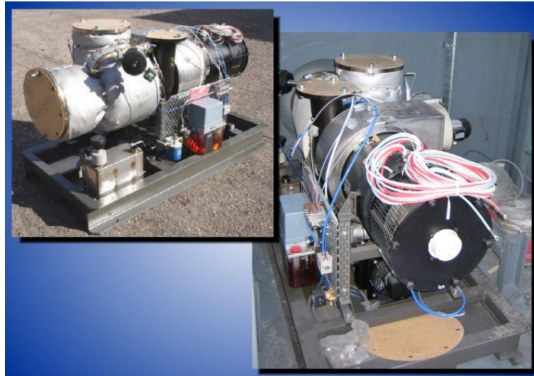
Fig. 21. A high speed micro turbine with permanent magnet (brushless) generator [31]
