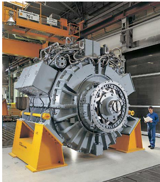
Fig. 19. Brushless DC submarine electric motor Permasyn [27]
