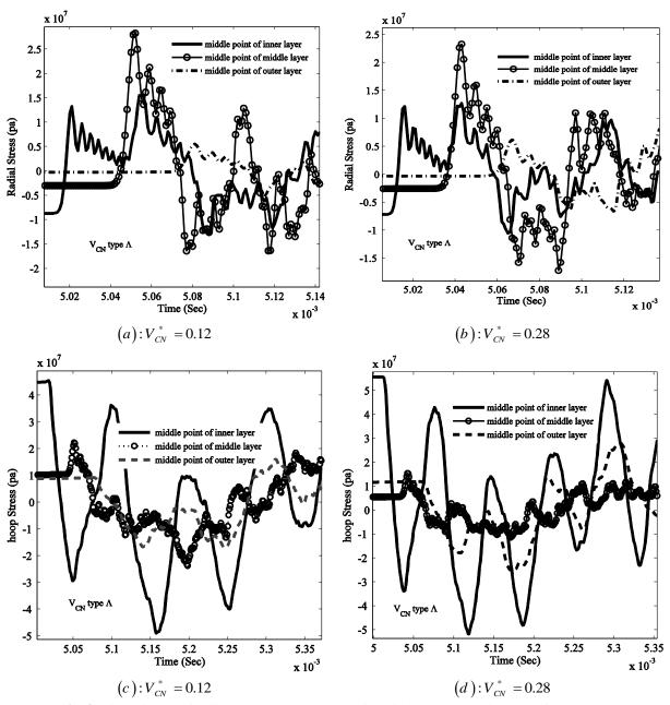
Fig. 8. Time history of radial stress and hoop stress for middle point on thickness of each layer
