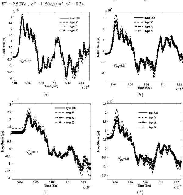
Fig. 5. Time history of radial stress and hoop stress for the middle point of cylinder thickness for various grading patterns of  $V_{\it CN}$
