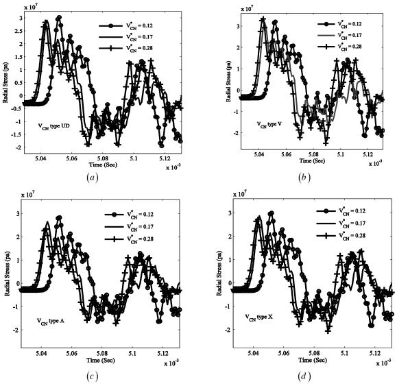
**Fig. 6.** Time history of radial stress at middle point of cylinder thickness for various values of  $V_{CN}^*$
