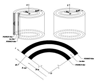
Fig. 4. Cylindrically layered structure with three layers
