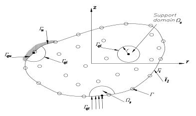
Fig. 2. Local domains used in the MLPG method
