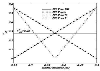
Fig. 1. Four types of variation of nanotube volume fraction  $(V_{CN})$  along the radial direction
