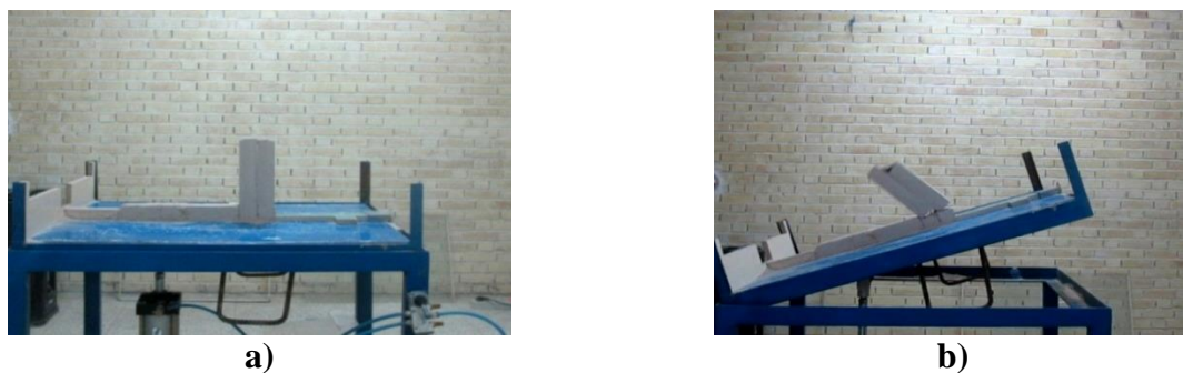
Fig. 8. Physical modeling of two-blocks with a potential of block-flexural toppling failure
