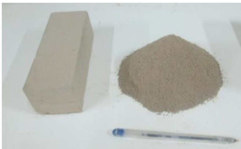
Fig. 2. Material used for physical modeling, before and after consolidation
