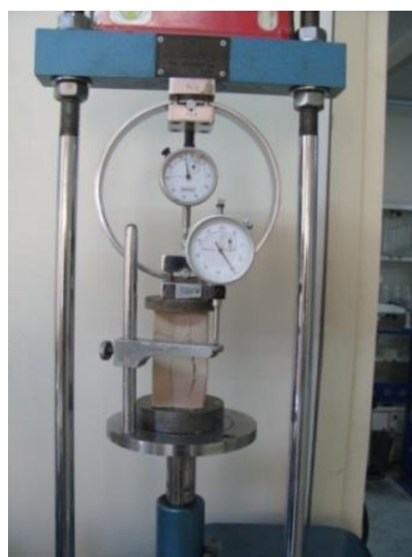
Fig. 3. Determination of the uniaxial compressive strength of the solid blocks
