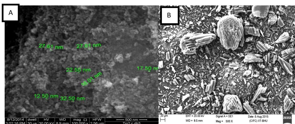
Fig. 4. Scanning electron micrograph (A) TiO<sub>2</sub>/Activated carbon nanocomposite (B) activated Carbon
