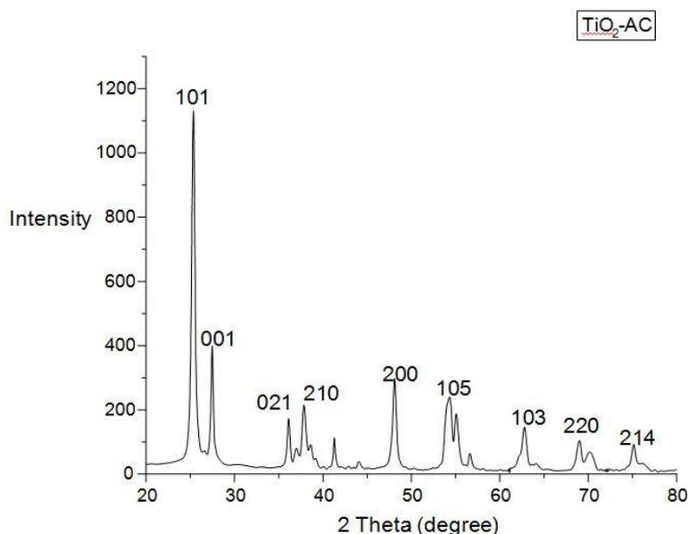
Fig. 3. XRD patterns of TiO<sub>2</sub>/Activated carbon nanocomposite
