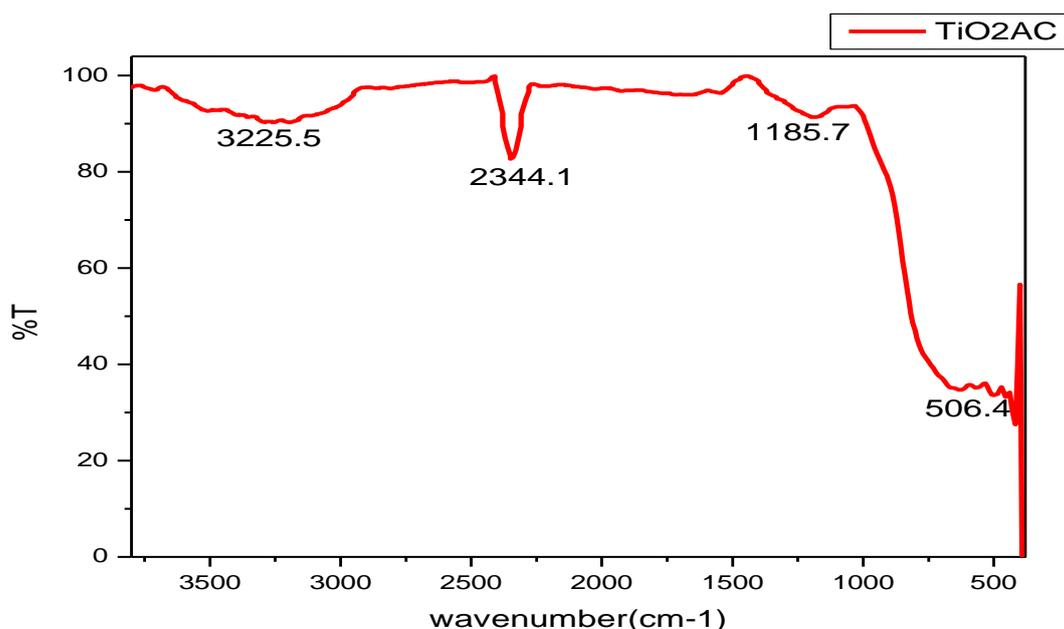
Fig. 5. FT-IR spectra of TiO<sub>2</sub>/Activated carbon nanocomposite
