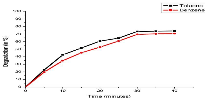
**Fig. 6. Degradation of benzene and toluene with respect to time in presence of TiO<sub>2</sub>/Activated carbon nanocomposite**
