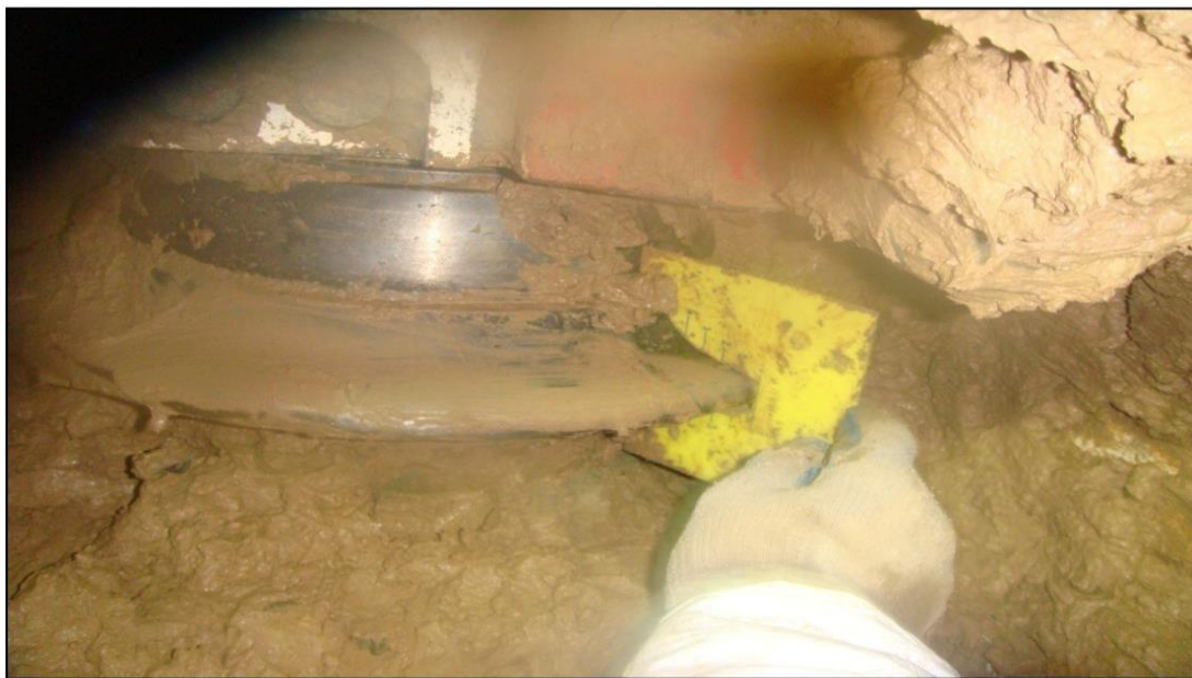
Fig. 7. The template fabricated for measuring machine cutting tools abrasion
