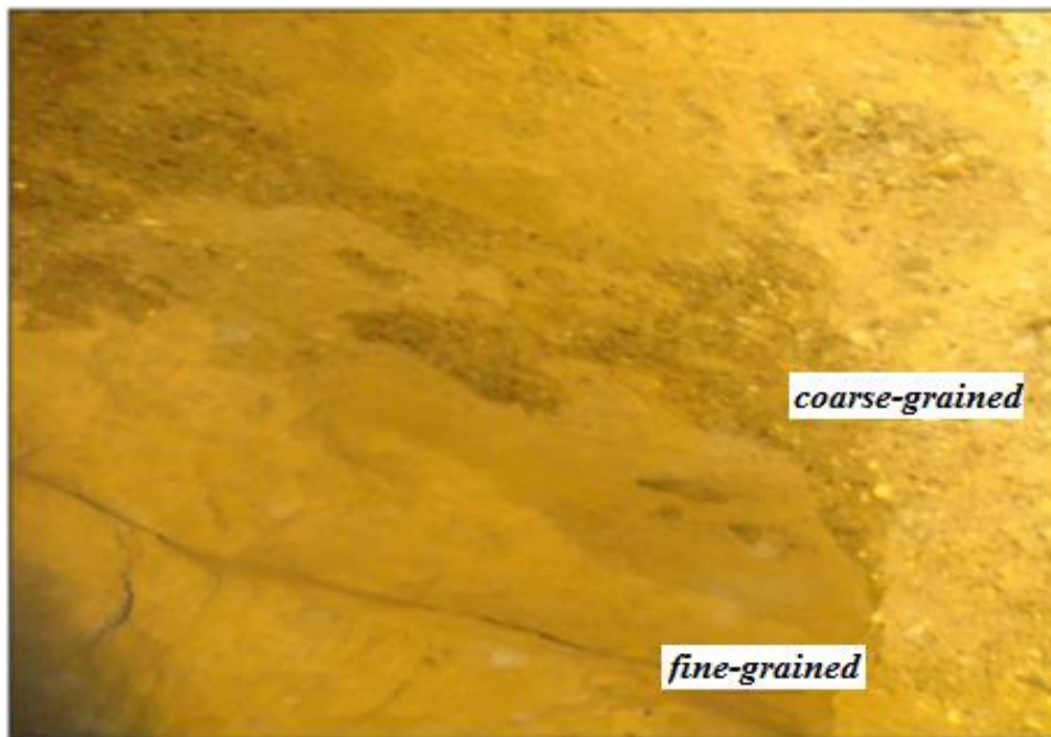
Fig. 12. Illustrates the extent of heterogeneity experienced at the tunnel face in the distance range (1152 to 1367 m) studied
