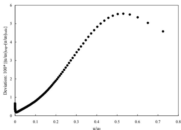
**Figure 3.** Deviation of 200 data points for R152a refrigerant calculated by new general model.
