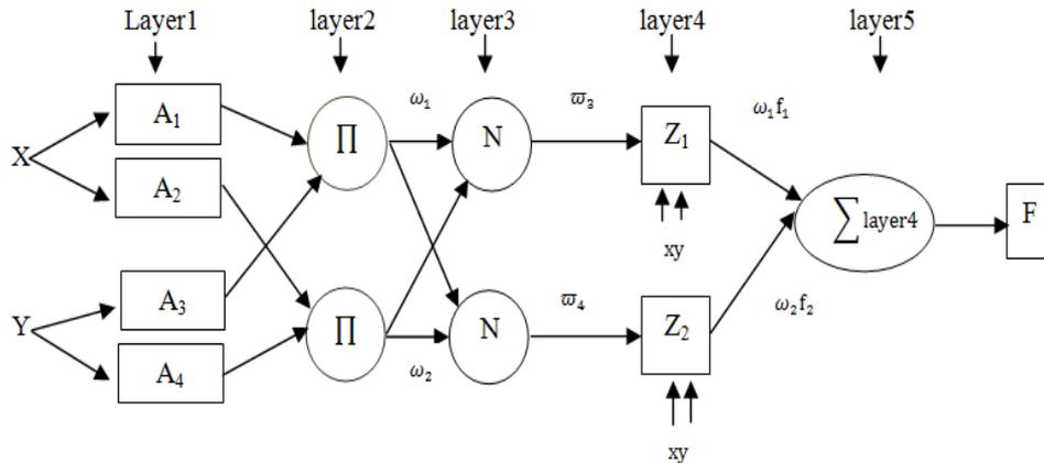
Fig. 1. Adaptive neuro-fuzzy inference system structure
