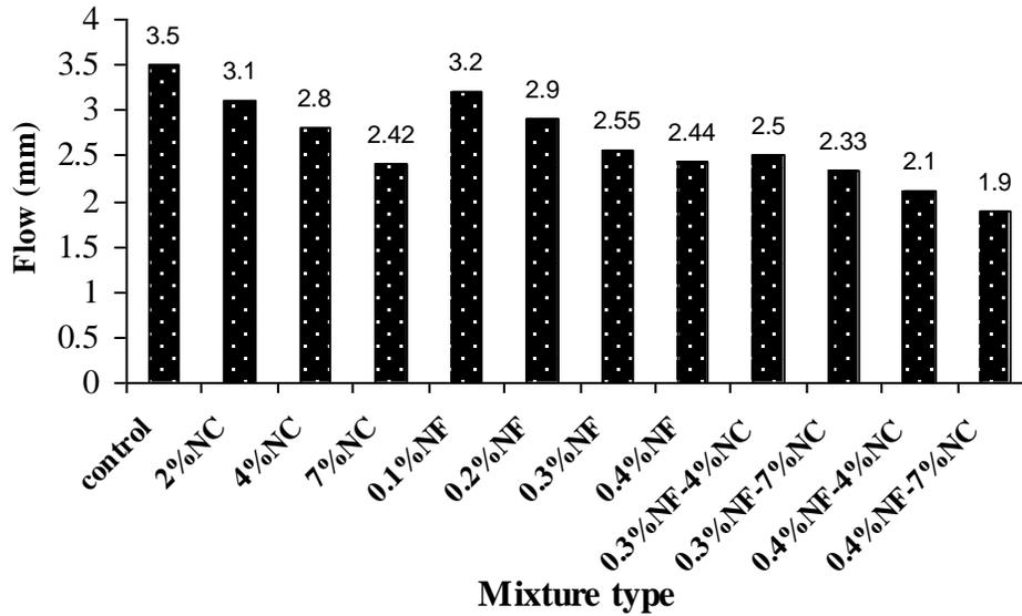
Fig. 4. Flow of the mixtures
