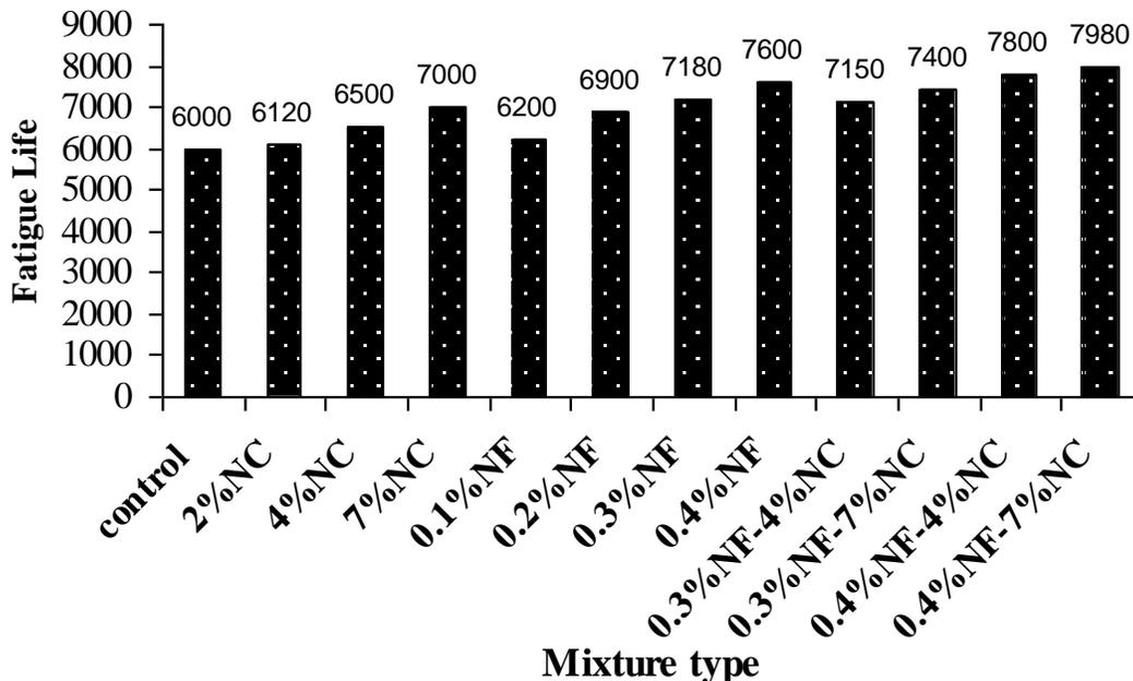
Fig. 8. Fatigue tests results
