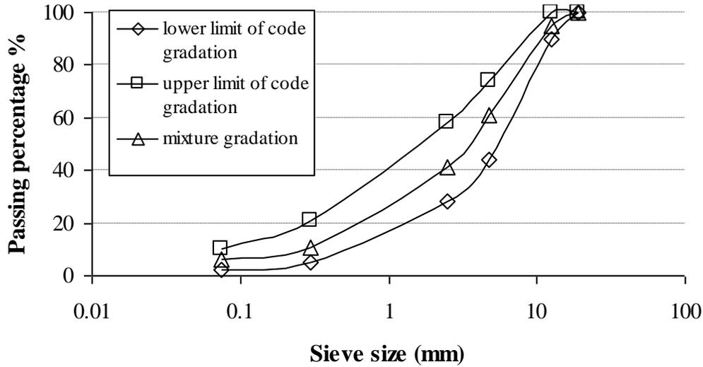
Fig. 1. Gradation of the mixture aggregates
