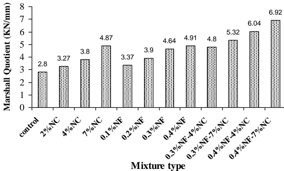
Fig. 5. Marshall Quotient of the mixtures
