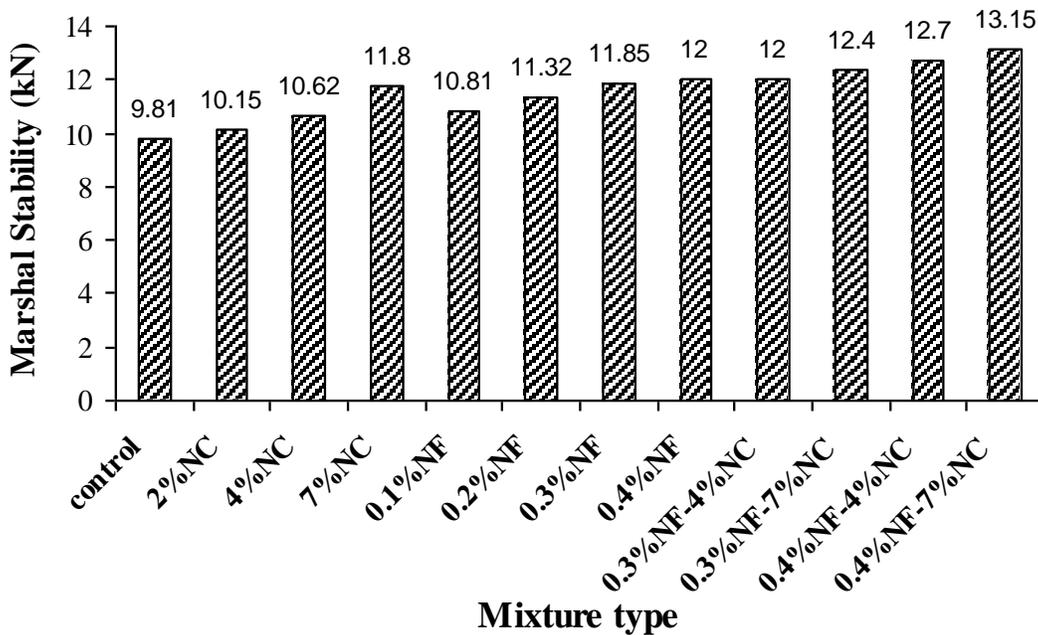
**Fig. 3.** Marshall Stability of mixtures
