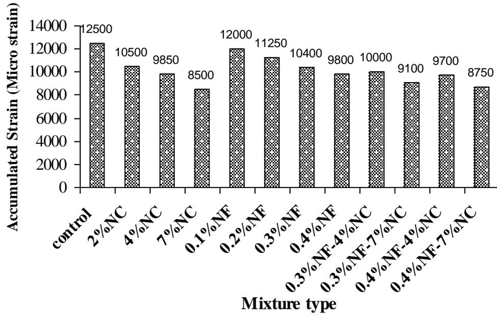
Fig. 7. Dynamic creep test results
