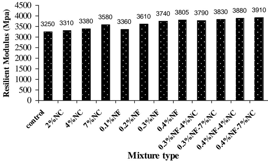
Fig. 6. Resilient modulus tests results
