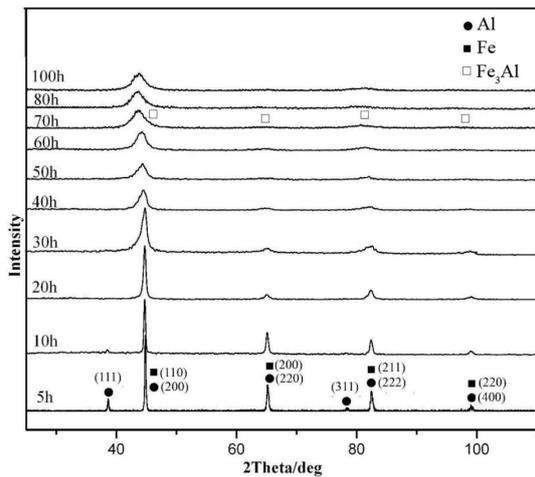
Fig. 2- XRD spectra of Fe-28 at.% Al powder after milling for different times.
