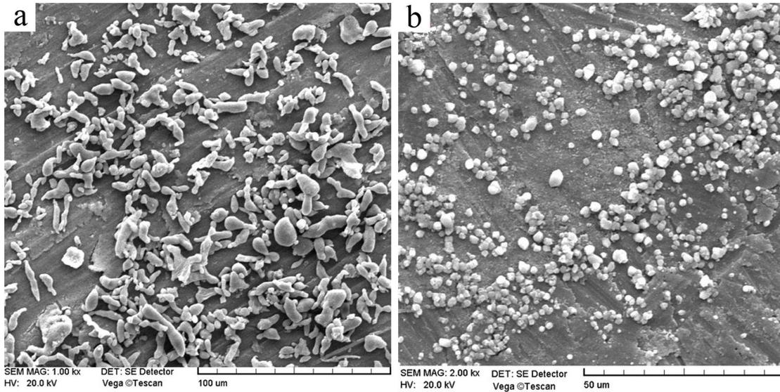
Fig. 1- SEM micrographs of pure powder of Al (a) and Fe (b).
