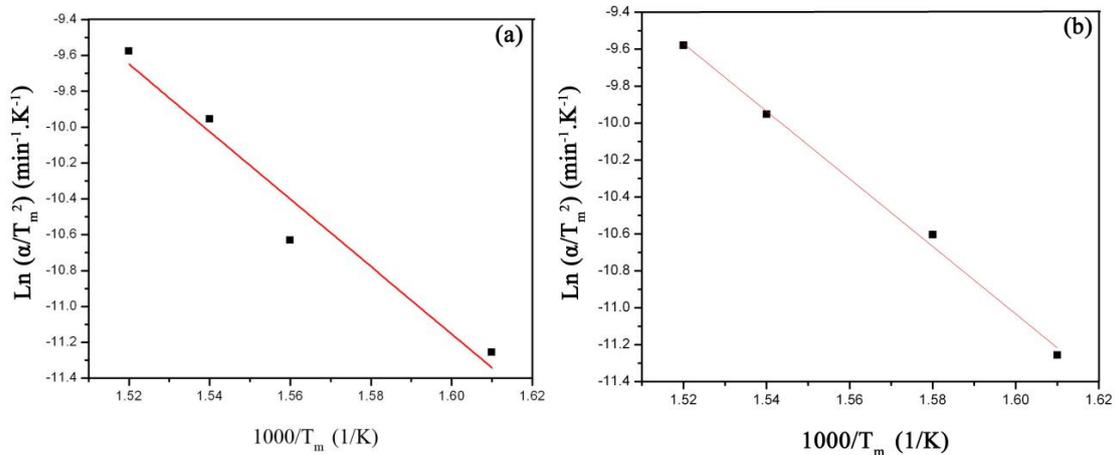
Fig. 9- Kissinger plots of DO3-type ordering in 70 (a) and 100 hours (b) milled Fe-28 at.% Al powder.
