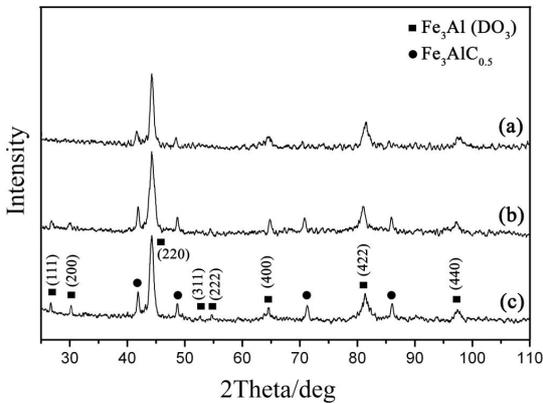
Fig. 7- XRD spectrums of Fe-28 at.% Al milled powder for different milling times of 40 (a), 70 (b) and 100 (c) hours after DSC heating.
