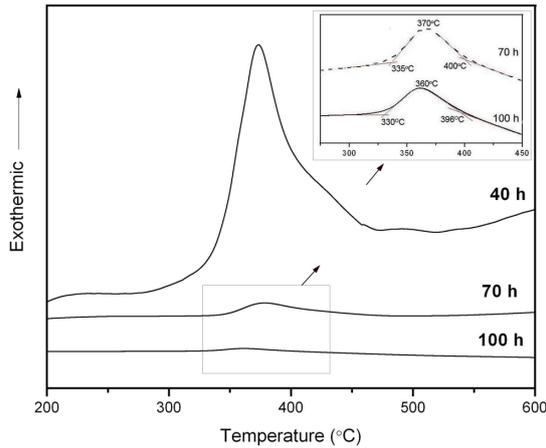
Fig. 6- DSC curves of the synthesized Fe-28 at.% Al powder in different milling times (heating rate: 10 K/min).
