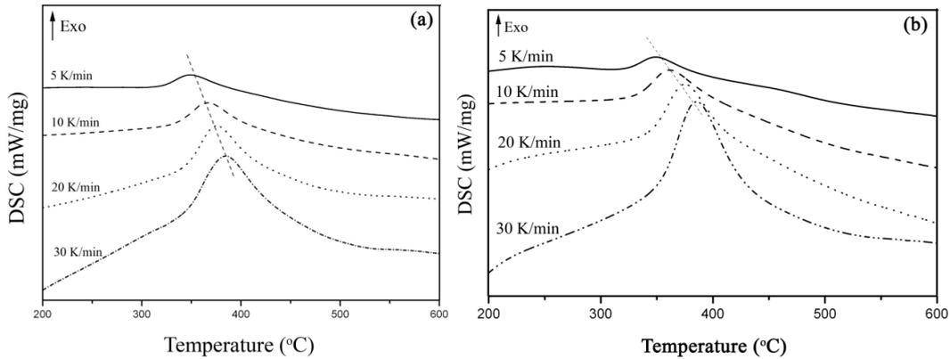
Fig. 8- DSC curves of the 70 (a) and 100 hours (b) milled Fe-28 at.% Al powder at different heating rates.
