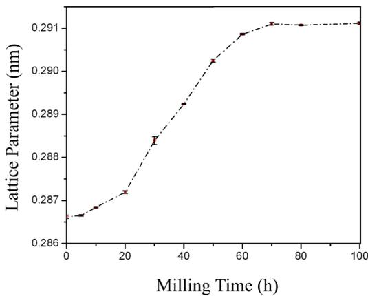
Fig. 3- The variation of lattice parameter of Fe-28 at.% Al powder as a function of milling time.
