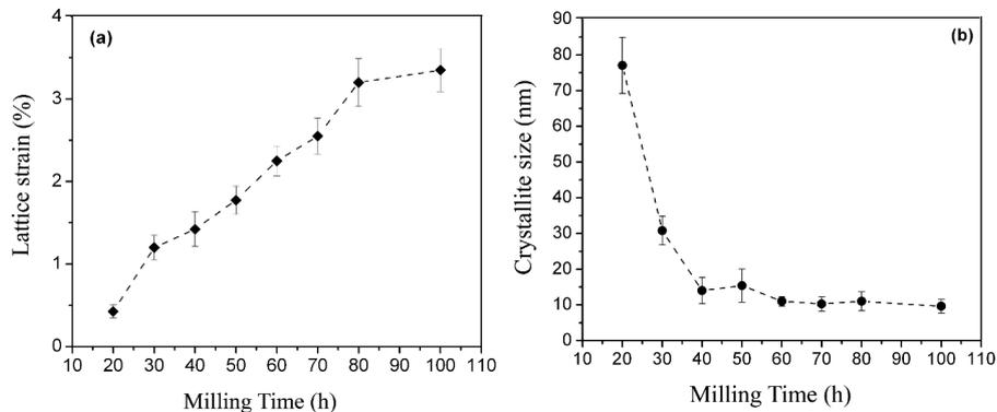
Fig. 4- Lattice strain (a) and average crystallite size (b) of the synthesized Fe-28 at.% Al powder as a function of milling time.
