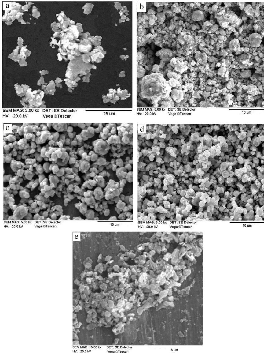
Fig. 5- SEM micrographs of Fe-28 at.% Al powder after 10 (a), 20 (b), 30 (c), 50 (d) and 70 (e) hours milling.
