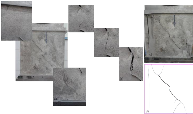
Figure 21. Specimen U30 ( \theta=45^\circ ) a) before test and initiation of outer crack tips b) crack coalescence in the bridge area c) after test d) schematic view of the propagated cracks.
