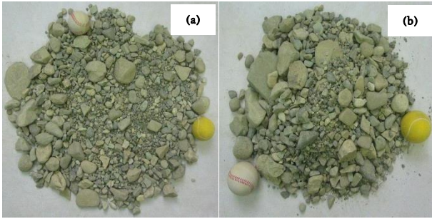
Figure 1. Laboratory sample of crushed rock (n=14, d 50 =19), (a): Pile (b): Distributed.
