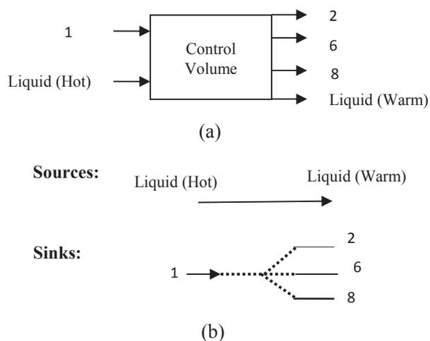
Figure 5. Simplified low capacity MED: a) System control volume; b) Sink & source flows.
