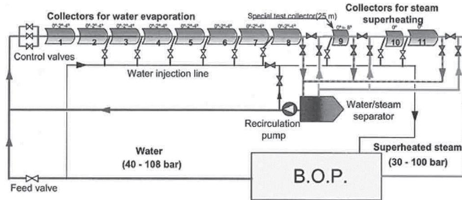
Figure 4. DISS loop schematic diagram, [13].
