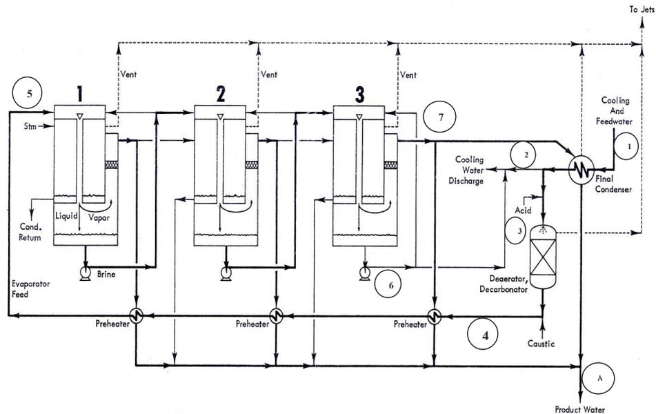
Figure 2. High capacity MED.
