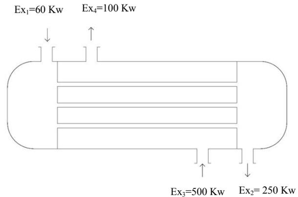
Figure 1. Schematic of a heat exchanger.
