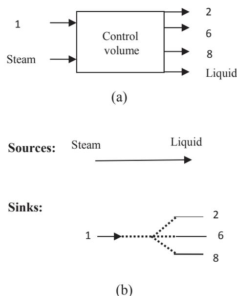
**Figure 3.** Simplified high capacity MED: a) System control volume; b) Sink & source flows.
