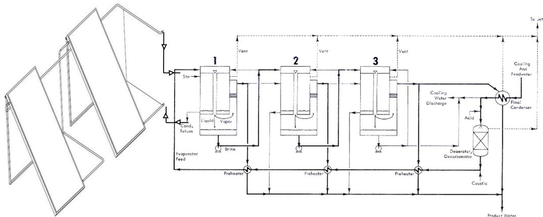
Figure 6. Solar water heating system of low capacity desalination system, input utility fluid temperature: 150°C.
