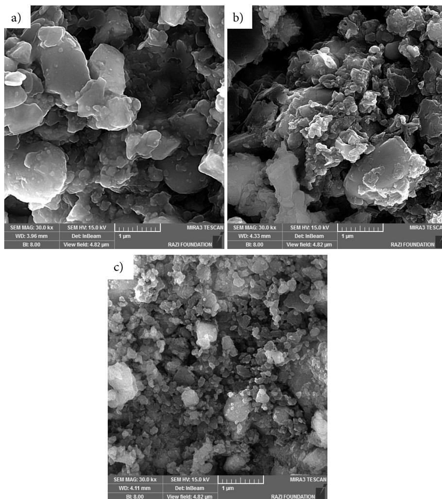
Fig. 2- SEM micrographs of the Mg-NiO for different milling time (the as-milled samples). (a) 15 minutes milling, (b) 30 minutes milling and (c) 60 minutes milling.
