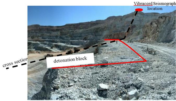
Fig. 2. Field location of the blasting block and the position of the related seismographs.
