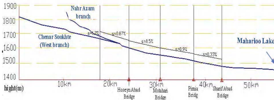
Fig. 3. The longitudinal section of the river passing through the city. In this Fig. existing bridges are seen. The total length of the river is 62 km and according to the report of Haseb Counseling Engineers (2004), the slope of river is changing between 0.33 and 1.2%
