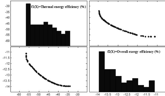
Figure 5. Results for thermal energy efficiency and overall exergy efficiency as objective functions in Pareto area
