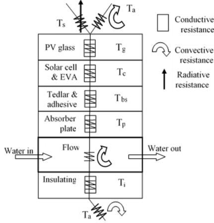
Figure 1. Thermal resistance circuit diagram of PV/T [7]
