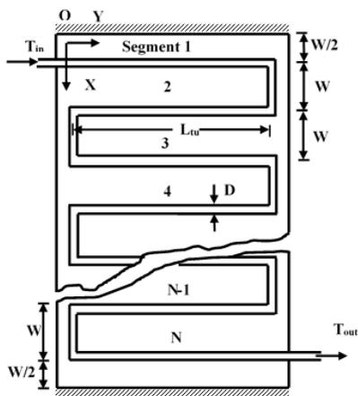
Figure 2. Schematic diagram of absorber plate and serpentine tube [11]
