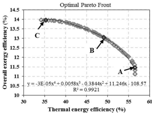
Figure 6. Pareto graph for thermal energy efficiency and overall exergy efficiency as objective functions
