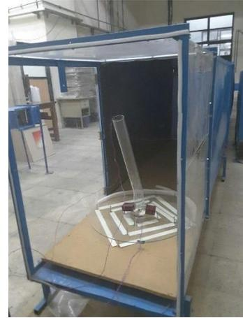
Figure 3. Experimental setup for Floating Solar Chimney located at the test section of a low speed wind tunnel
