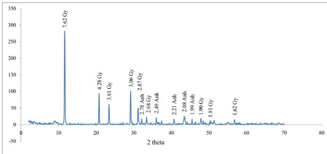
Figure 5. X-ray diffraction patterns of secondary gypsum from with minor anhydrite content from the Tang-e- Geltorsh Section. Gy: gypsum; Anh: anhydrite.
