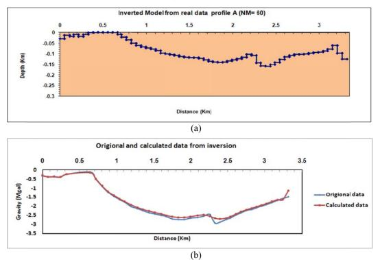
**Figure 11.** Produced model (60 model parameters) from the inversion using damping term (a), and the gravity response of the inverted model together with the real one data (b), along profile A.
