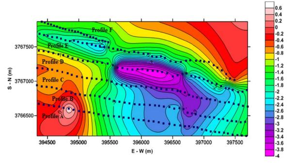
Figure 6. 2-D Bouguer gravity anomaly (mGal) together with the position of the stations and the profiles.
