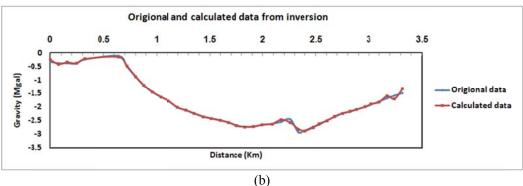
**Figure 9.** Produced model (40 model parameters) from the inversion (a) and gravity response of the inverted model together with the real gravity data (b), along profile A.
