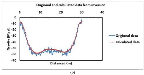
**Figure 3.** Result of the inversion of synthetic noisy gravity data (a), comparison of the observed and calculated gravity data (b).
