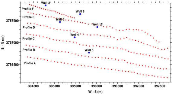
Figure 7. Positions of excavated drinking water wells on the measured gravity data profiles map.
