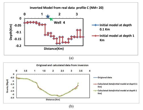
**Figure 12.** Produced model (20 model parameters) from the inversion (a), and the gravity response of the inverted model together with the real one data (b), along profile C.
