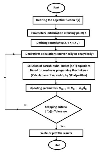
Figure 1. Flowchart of the non-linear constrained optimization algorithm.
