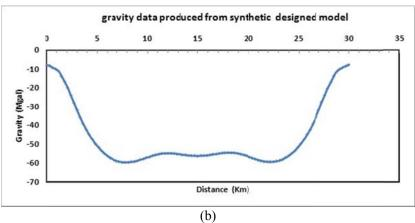
**Figure 2.** Designed synthetic model composed of 40 elementary prisms whose bottoms make interface between basement and sediments (a). Gravity response of the synthetic model (b).
