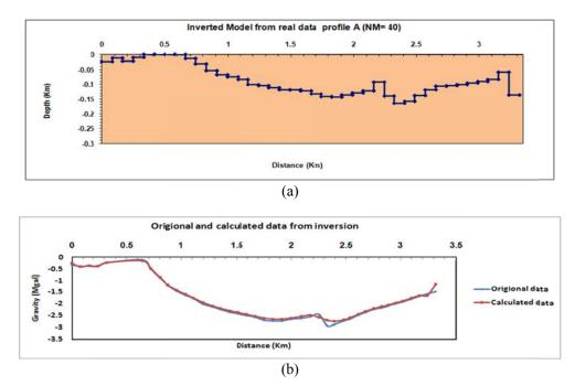
**Figure 10.** Produced model (40 model parameters) from the inversion using damping term (a), and gravity response of the inverted model together with the real gravity data (b), along profile A.
