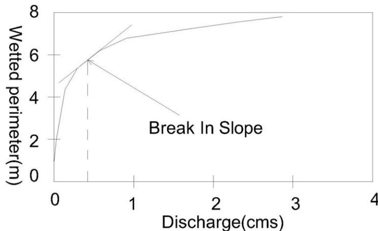
**Fig. 1.** Schematic view of wetted perimeter method (Gippel et al., 1998)
