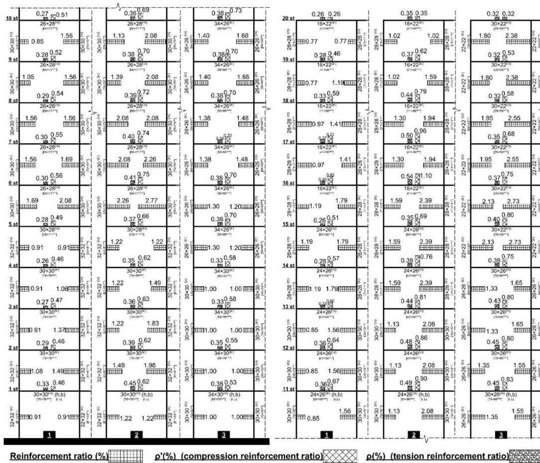
Fig. 9. Detail of design 20 story building in: 1) PBPD method with SSI effect, 2) PBPD method without SSI effect and 3) Strength based method
