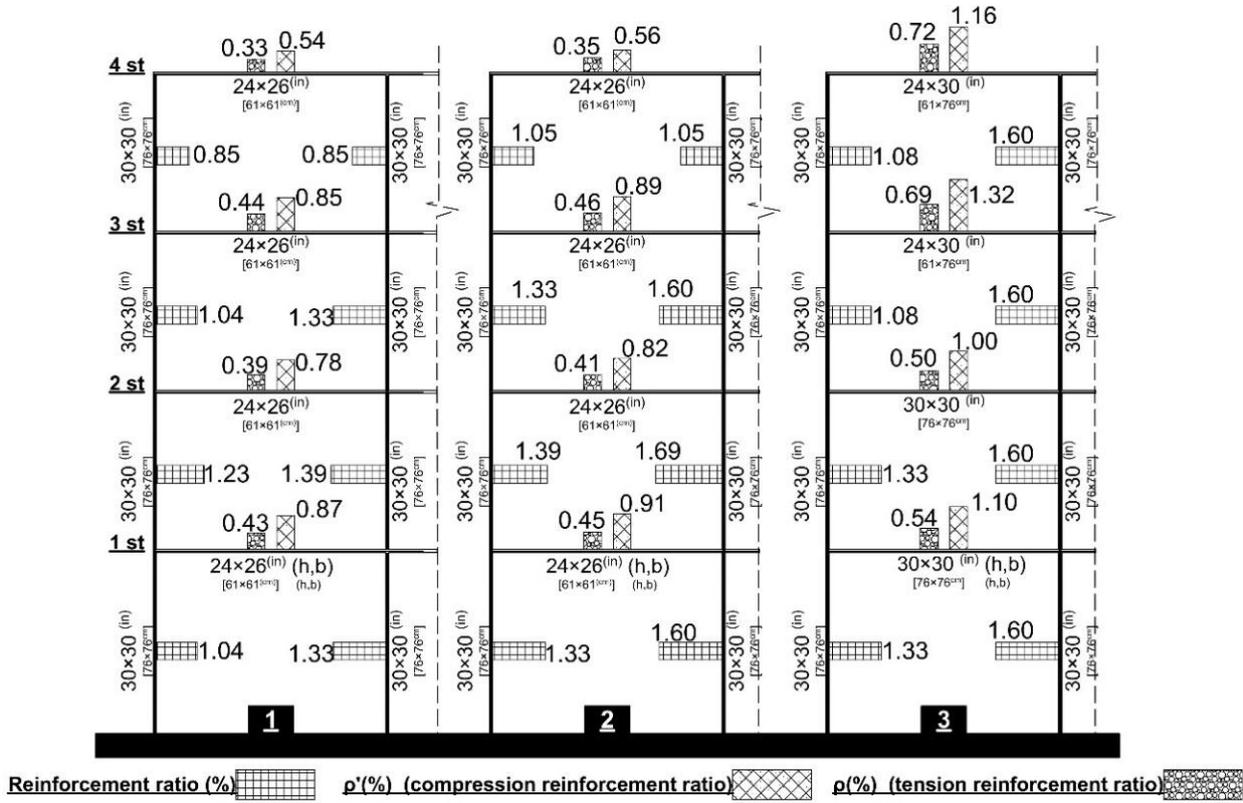
Fig. 6. Detail of design 4 story building in: 1) PBDP method with SSI effect, 2) PBDP method without SSI effect and 3) Strength based method
