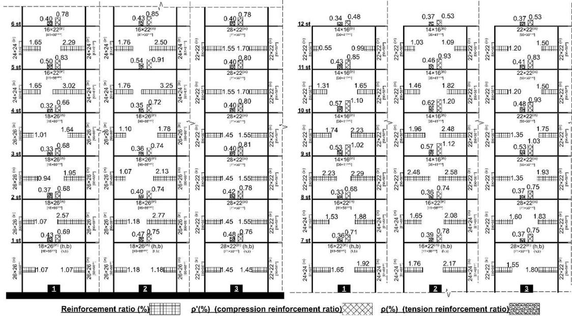
Fig. 8. Detail of design 12 story building in: 1) PBPD method with SSI effect, 2) PBPD method without SSI effect and 3) Strength based method
