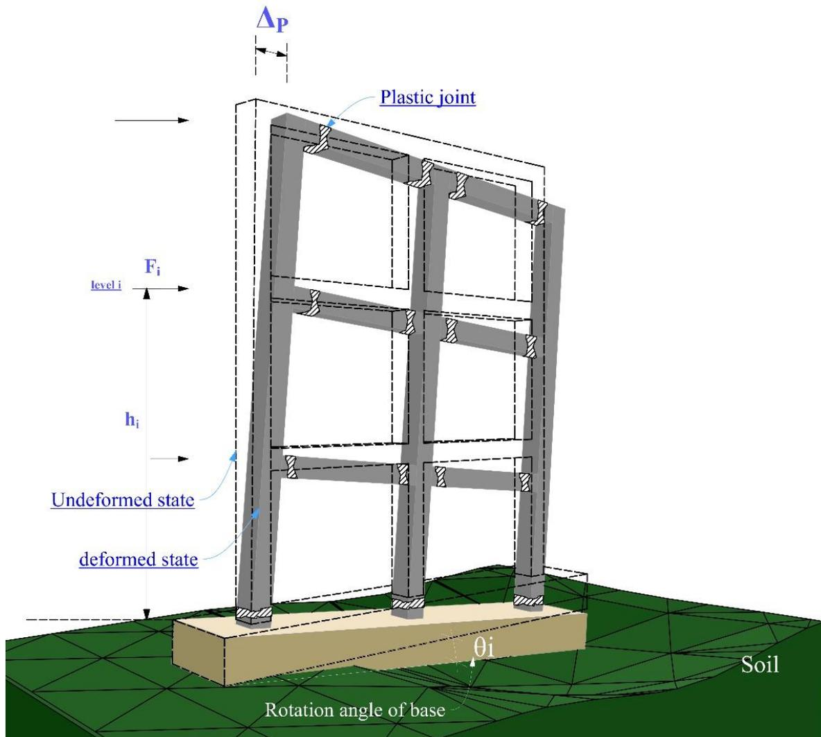
Fig. 2. The SSI effect in PBPD method
