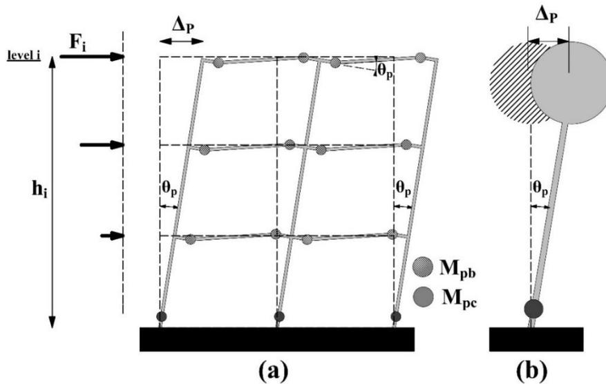
Fig. 1. a) The desired yielding mechanism of reinforcement concrete spatial moment frames, b) The equivalent single degree of freedom
