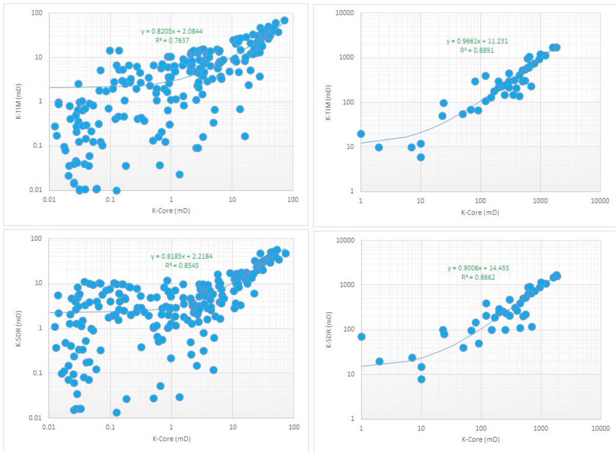
Figure 4. Correlation between predicted permeability from Timur-Coates and SDR models and those of core plugs. The Timur-Coates model in carbonate part has poorer correlation than the SDR model, whereas in clastic part it has greater correlation than the SDR model. Generally, the NMR log based permeability in the clastic parts (right) are more accurate than that of carbonate parts (left).
