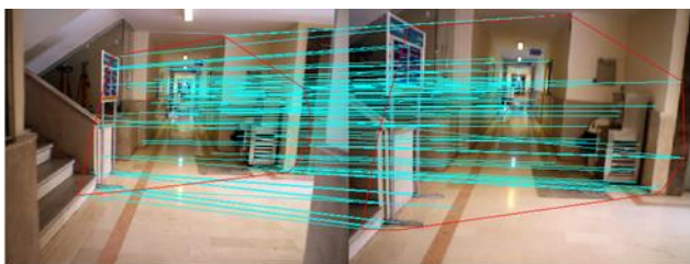
Figure 1. The separation of far from near obstacles in the algorithm of Al-Kaff et al. (2017)
