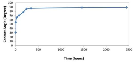
**Figure 3.** Contact angle measurements without sandpaper in a core slice at 50°C
