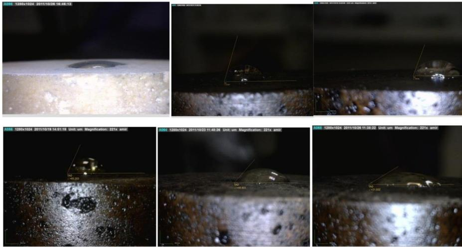
Figure 6. Contact angle measurements during oil aging
