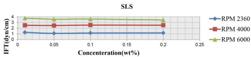
Figure 9. IFT vs. surfactant concentrations at different RPMs for SLS
