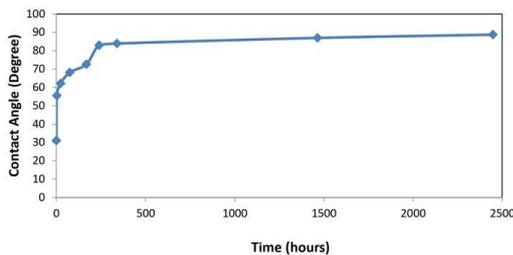
**Figure 1.** Contact angle measurements without sandpaper in a core slice at 25°C
