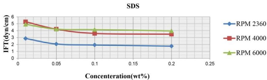
**Figure 11.** IFT vs. surfactant concentrations at different RPMs for SDS
