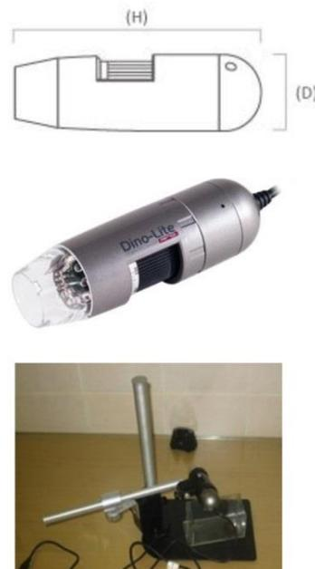
**Figure 5.** Schematic view of Dino-Lite Pro Microscope with 10cm (H) x 3.2cm (D) and 100g weight
