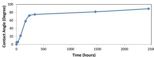
**Figure 2.** Contact angle measurements with sandpaper in a core slice at 25°C
