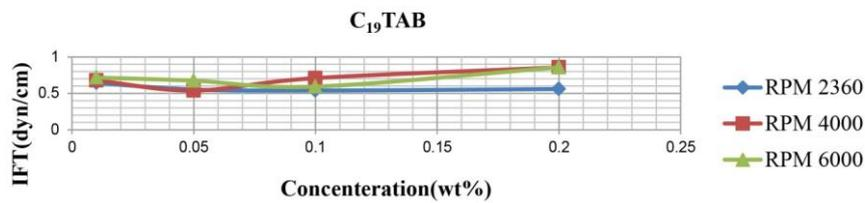
Figure 8. IFT vs. surfactant concentrations at different RPMs for C19TAB
