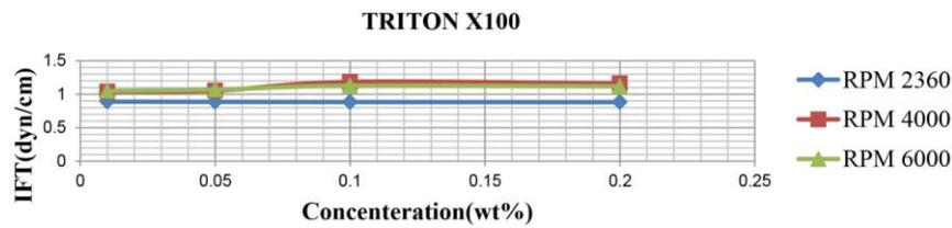
**Figure 10.** IFT vs. surfactant concentration at different RPMs for TRITON X100
