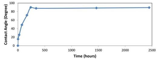
**Figure 4.** Contact angle measurements with sandpaper in a core slice at 50°C
