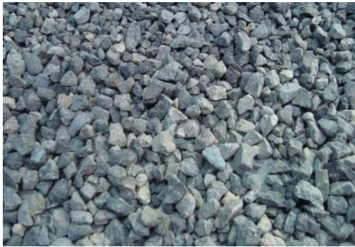
Fig. 3. Gravel for stone column.
