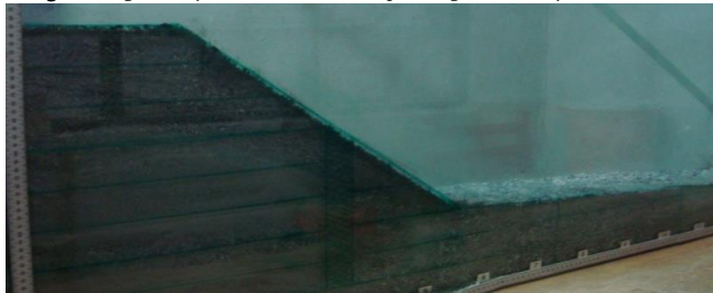
Fig. 8. The reinforced slope using an ordinary stone column.
