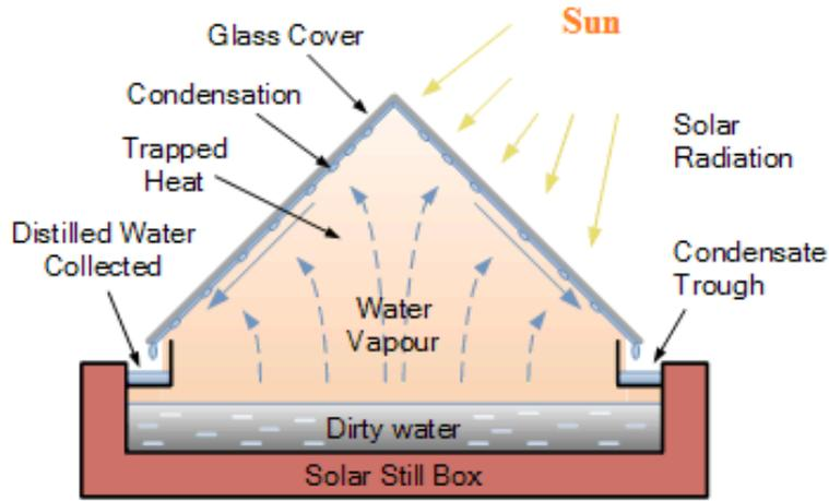
Figure 1. Solar still and its compartments
