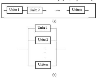
Figure 1. (a) A series production system; (b) a parallel production system
